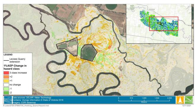
Figure 18 Change in flood hazard between existing and design – 1% AEP
