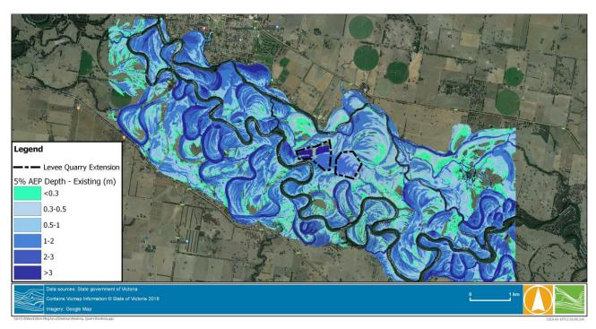
Figure 2-11 5% AEP flood depth
