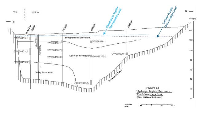
FIGURE 3-4 STYLISED CROSS SECTION ADJACENT THE PROPOSED QUARRY EXPANSION SITE (AFTER KULATUNGA 2009)
