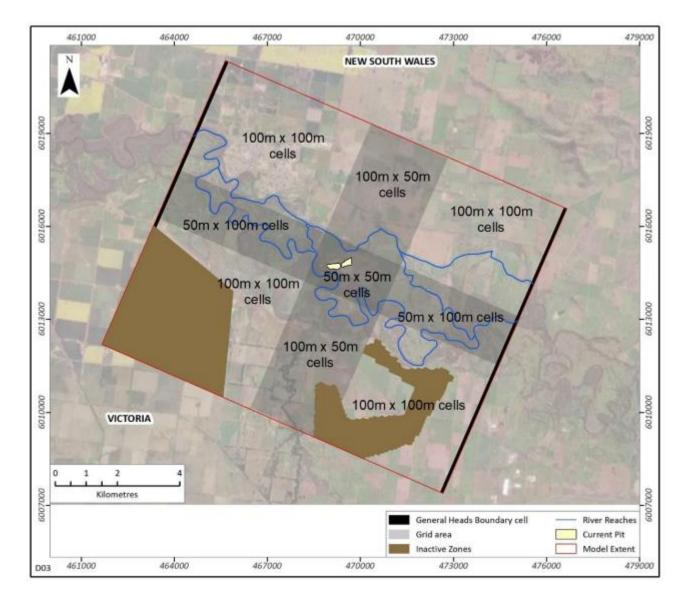
FIGURE 5-1 EXTENT OF NUMERICAL MODEL AND CELL DISCRETISATION (WATSEC ENVIRONMENTAL, 2022)
