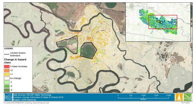
Figure 17 Change in flood hazard between existing and design – 5% AEP (warm colours indicate the flood hazard has increased, shades of green indicate the hazard is lowered under design conditions)
