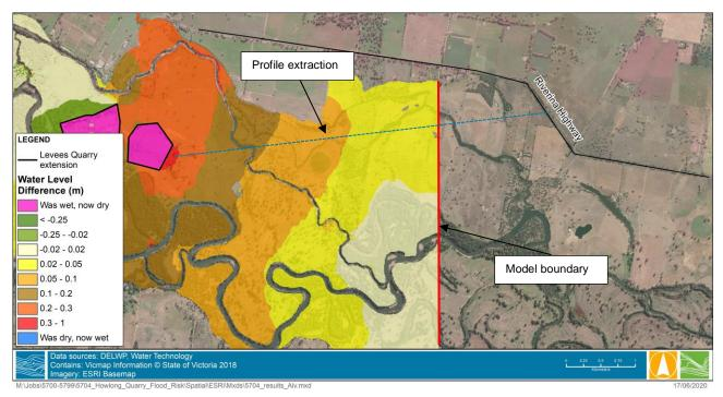
Figure 1-1 1% AEP flood difference map and upstream model boundary
