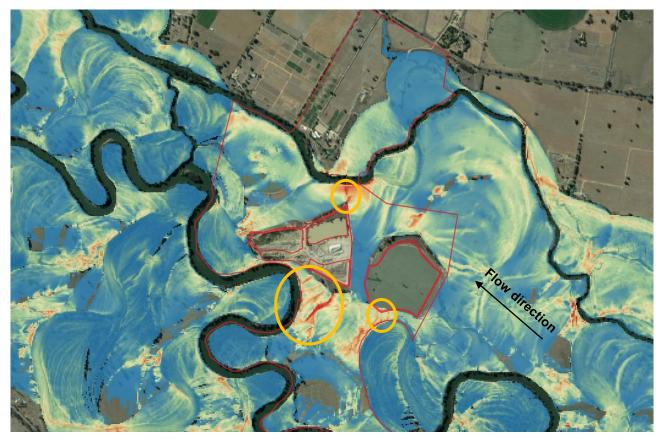
FIGURE 6 HYDRAULIC MODELLING OUTPUT INDICATING SHEAR STRESS ACROSS THE FLOODPLAIN DURING A 20% AEP FLOW EVENT FOR THE DEVELOPED CASE. THE KEY AREAS OF POTENTIAL EROSION ARE REPRESENTED BY THE ORANGE CIRCLES.
