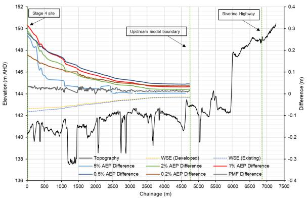
Figure 1-2 1% AEP water level profiles and water level changes for all design events from site to Riverina Highway
