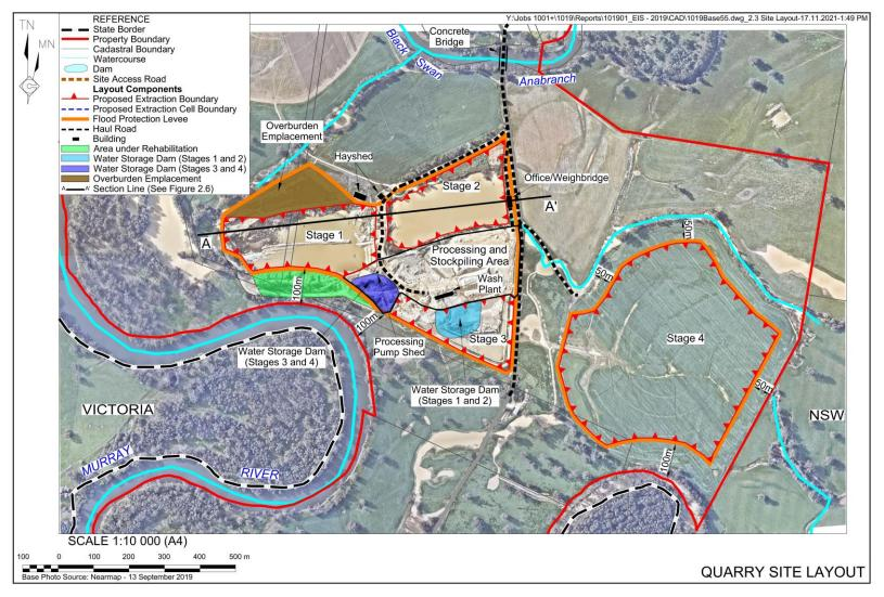
FIGURE 2 PROPOSED QUARRY EXTRACTION STAGES AND LEVEES AROUND THE EXTRACTION PITS (SHOWN IN ORANGE). IMAGE SUPPLIED BY R.W. CORKERY & CO. PTY LIMITED.
