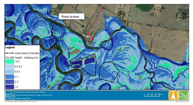
Figure 2-10 5% AEP flood depth at site
