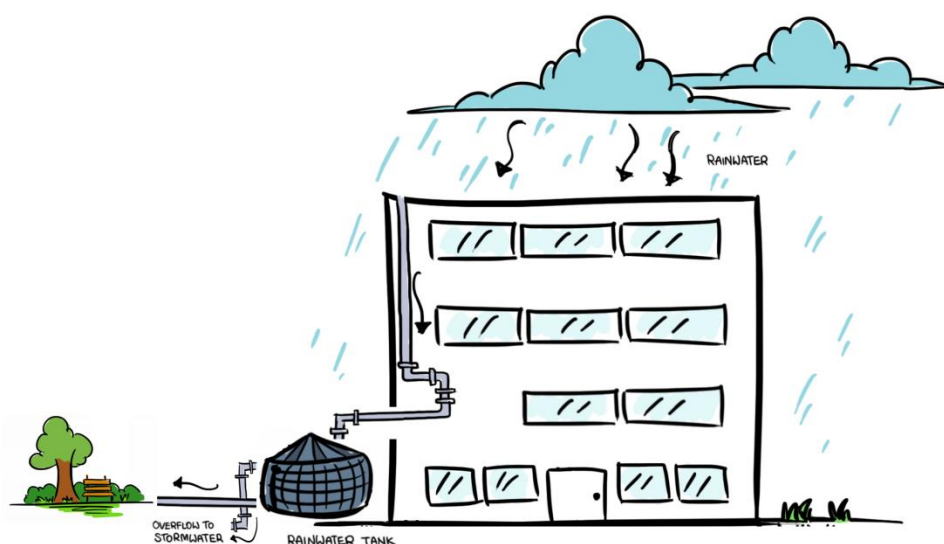
Figure 3: Rainwater harvesting system for landscape irrigation
