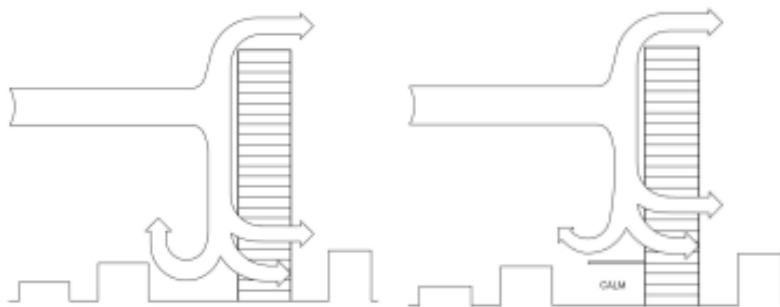
Figure 6: Canopy Windbreak Treatment. (L) Downwash to street level may generate windy conditions for pedestrians. This is particularly true for buildings much taller than the surrounding buildings. (R) A large canopy is a common solution to this pedestrian-wind problem at street level.
