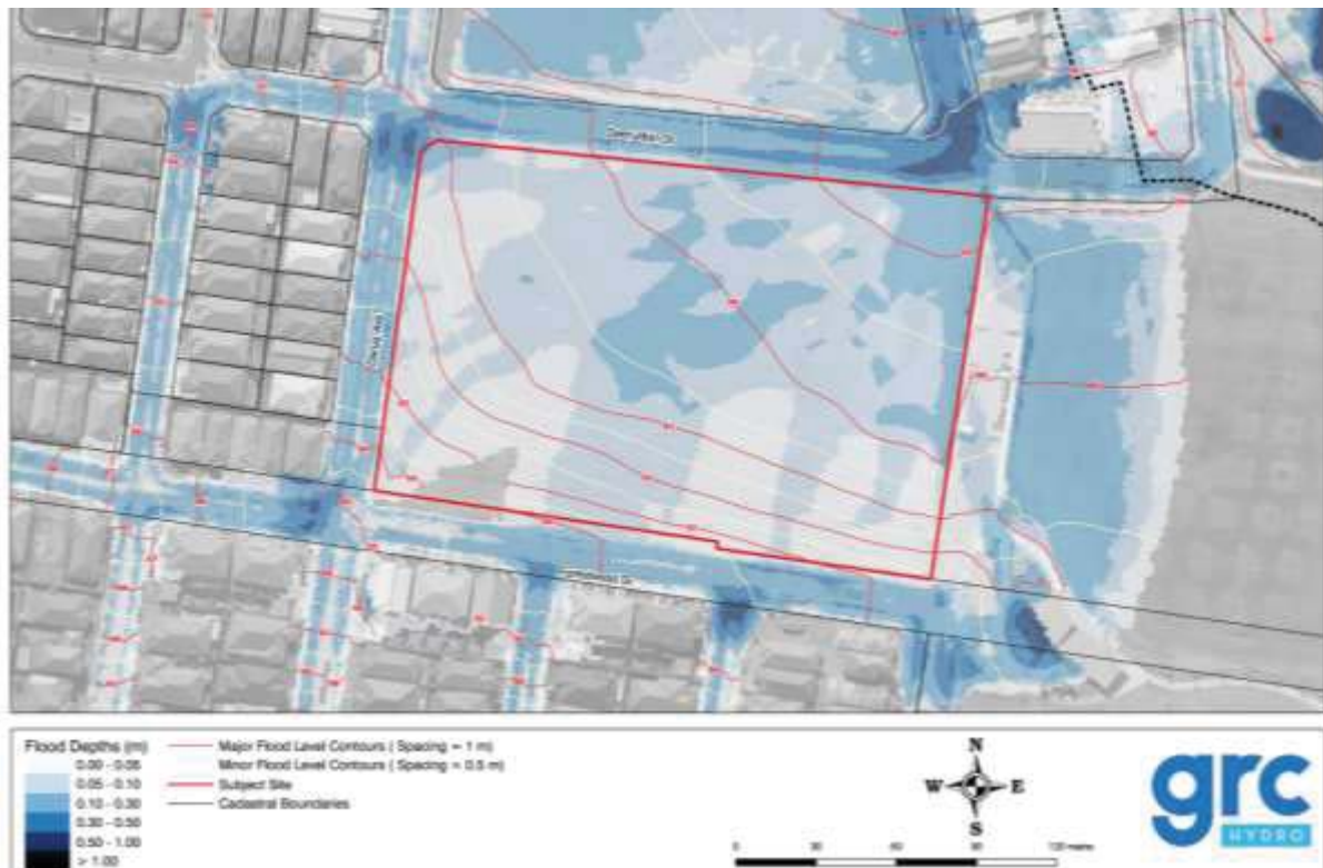
Figure 4 – PMF Pre-developed flood mapping (extract from Overland Flow Flood Study )
