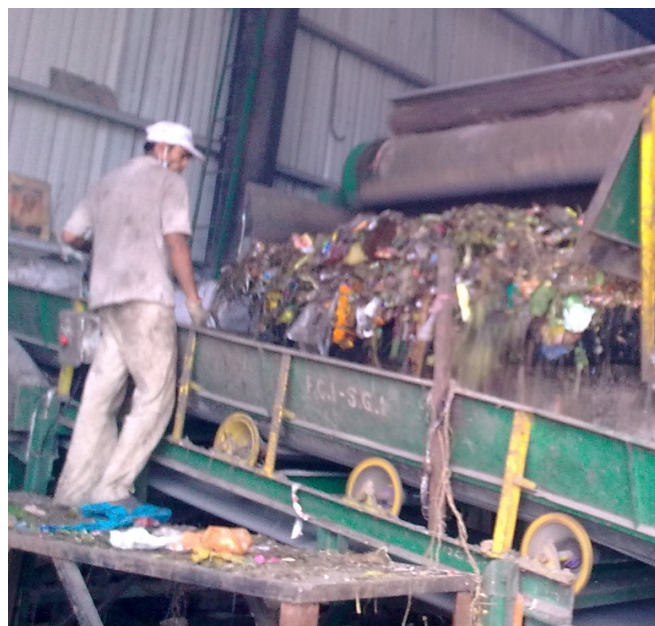
A worker manually separates large objects from the conveyor at Hanjer Biotech Energies Ltd. in Nagpur, India. This is done to prevent damage to the machinery. (Photo: GAIA)
