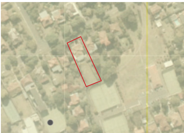
Figure 2.23 1986 aerial image with 37 Bancroft Avenue outlined in red. The rear skillion roof wing appears to have a bigger, rectangular footprint. Source: NSW Government Historical Imagery Viewer
