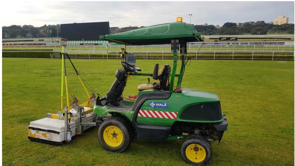
Figure 3: MALA 400MHz 3D MIRA acquiring data on site.
