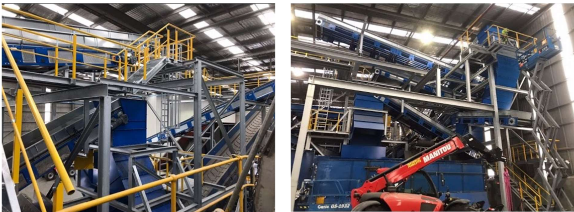
Figure 2.2. MRF layout at Visy Smithfield showing elevated plant platforms connected by walkways and stairs for access and conveyors for material transport.
