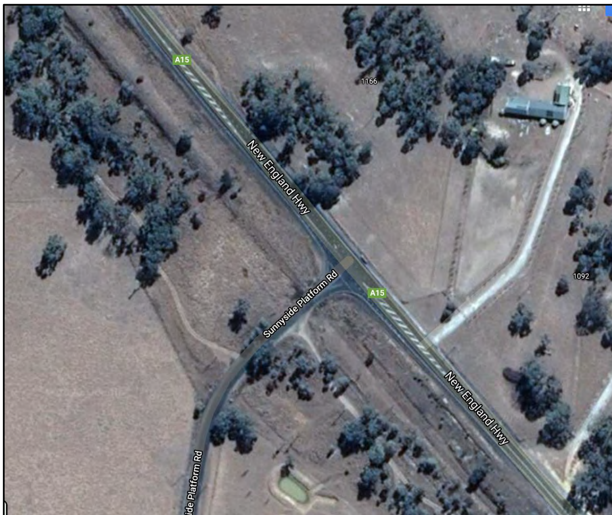
Figure 2-1– aerial photo showing layout of New England Highway and Sunnyside Platform Road showing straight alignment of New England Highway and sheltered turn lane (source: google maps).
