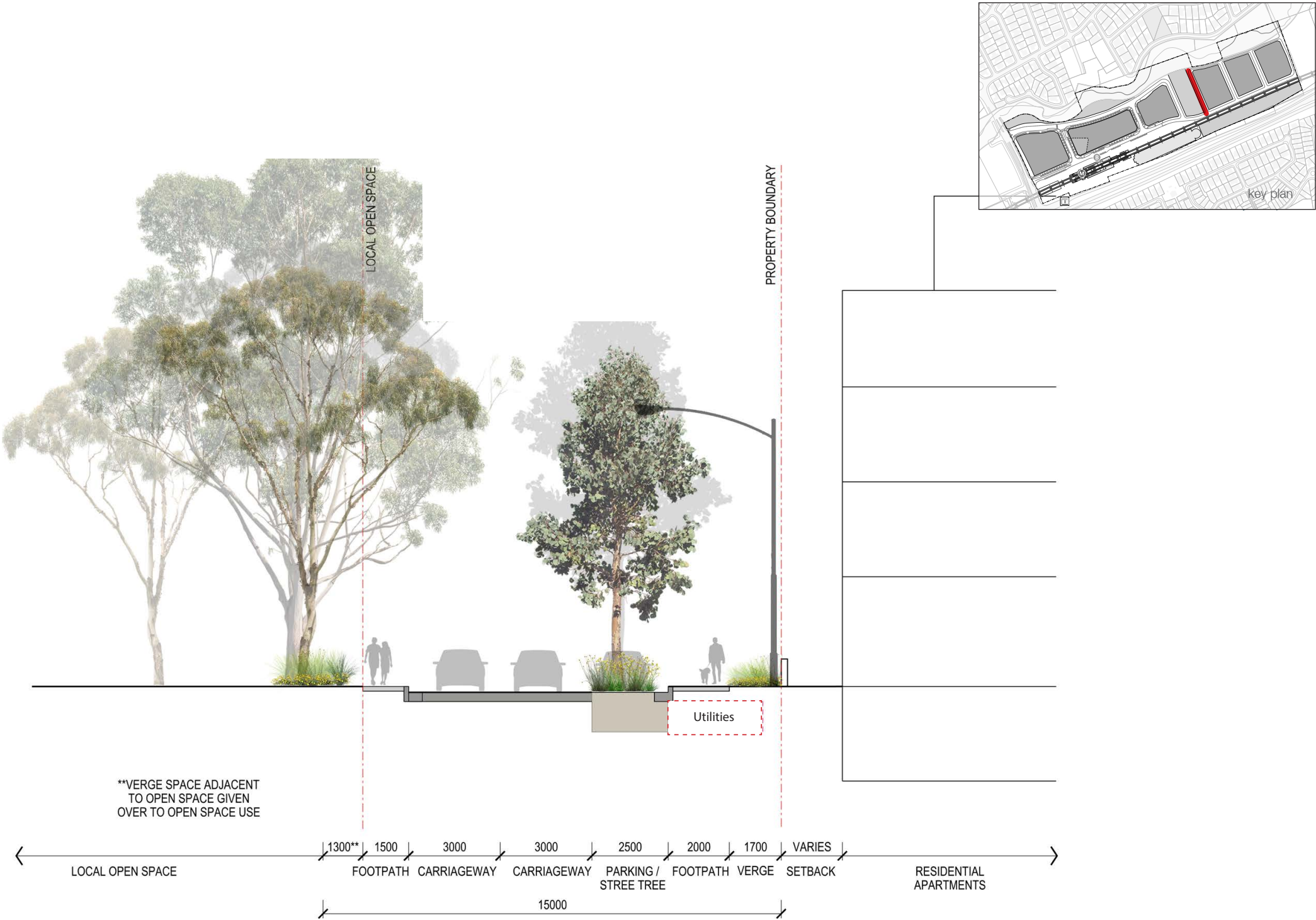
Figure 40: Local street cross section - adjacent to the Local Urban Park
