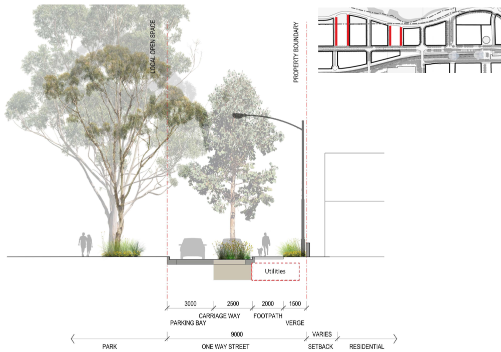
Figure 4.2.8.6 Local Street Section 06
