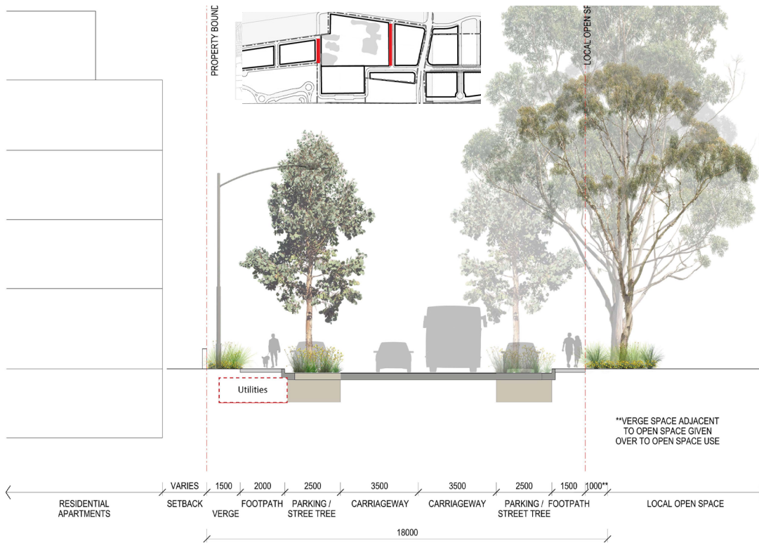
Figure 4.2.8.3 Local Street Section 03
