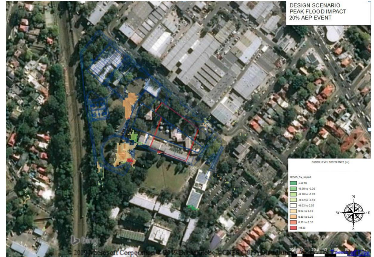
Figure 15. 20% AEP event flooding impact
