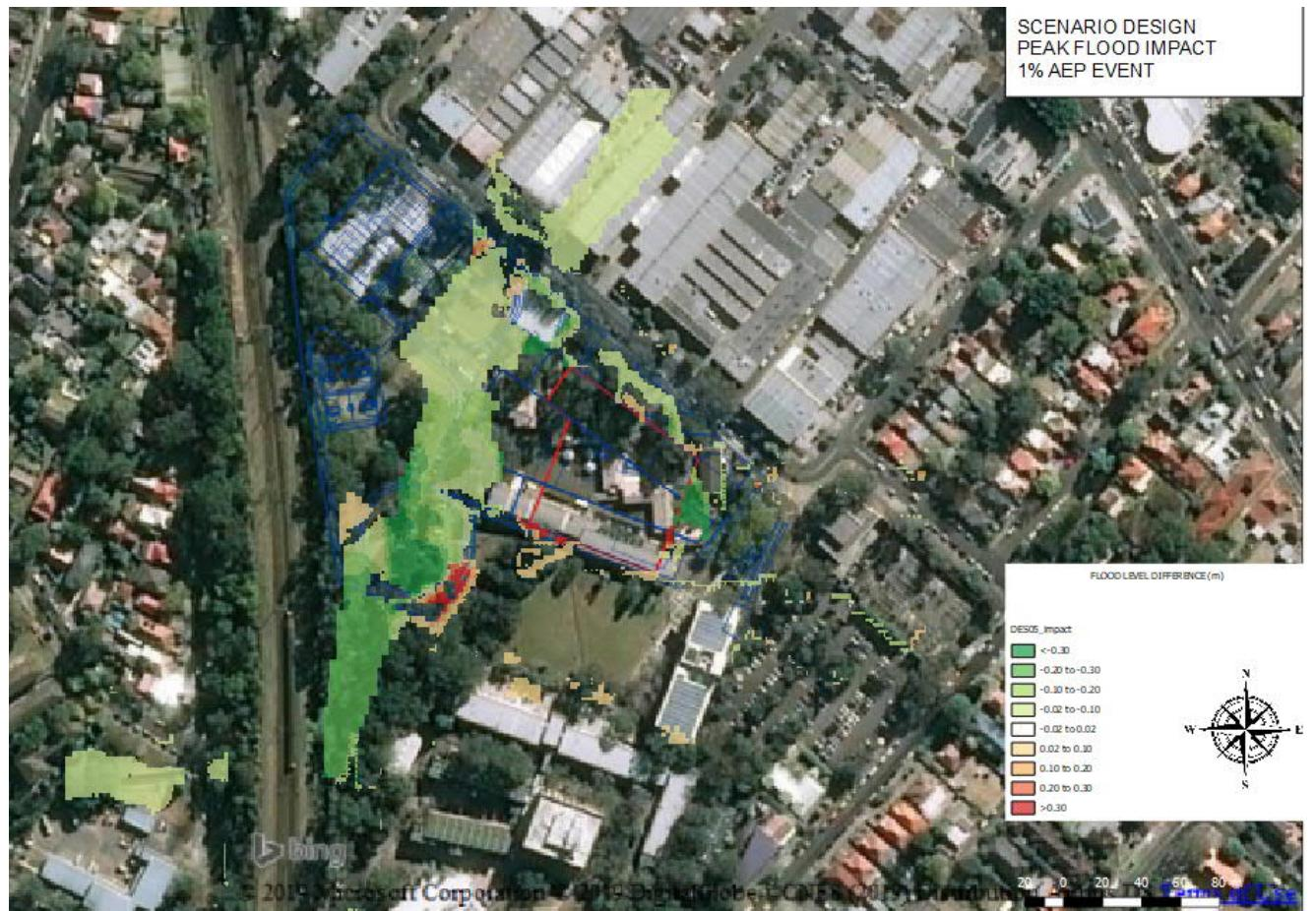
Figure 16. 1% AEP event flooding impact
