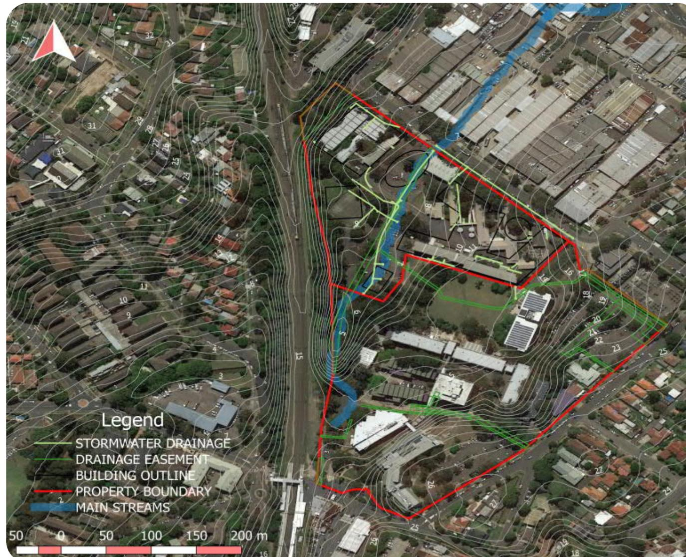
Beyond the subject site, but within the Meadowbank TAFE site, this trunk discharges into an overgrown, partially concrete lined, creek as shown in Figure 4.
