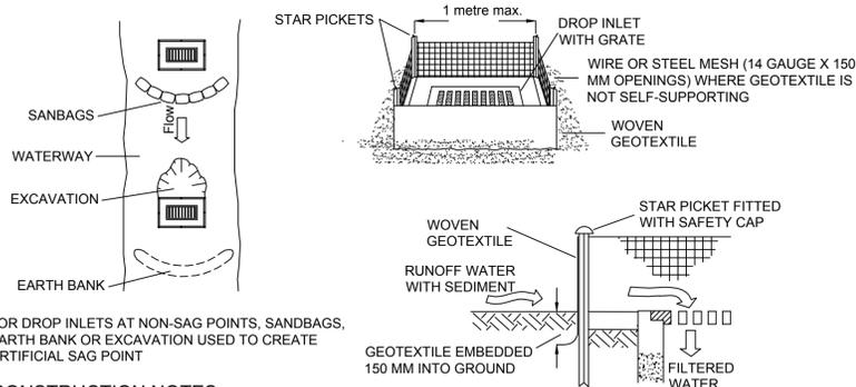
FOR DROP INLETS AT NON-SAG POINTS, SANBAGS, EARTH BANK OR EXCAVATION USED TO CREATE ARTIFICIAL SAG POINT
