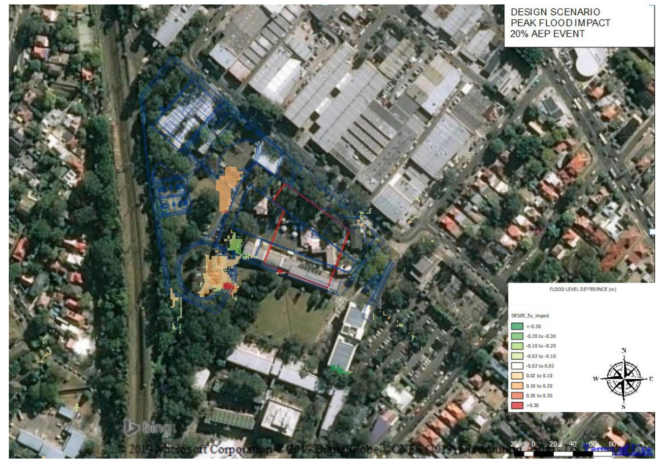
Figure 15. 20% AEP event flooding impact
