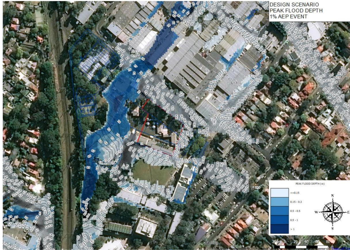
Figure 13. Overland flooding under post-development conditions for 1% AEP event
