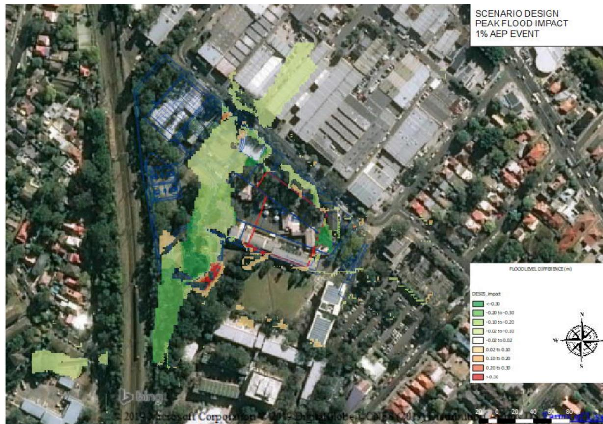
Figure 16. 1% AEP event flooding impact
