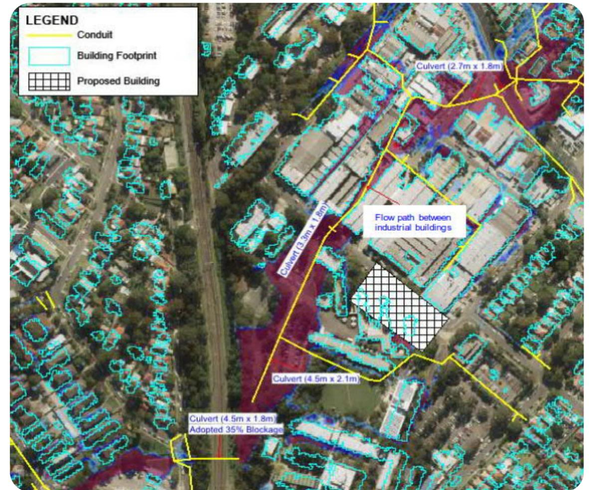
Figure 6. Key drainage structures (Source: ARUP)
