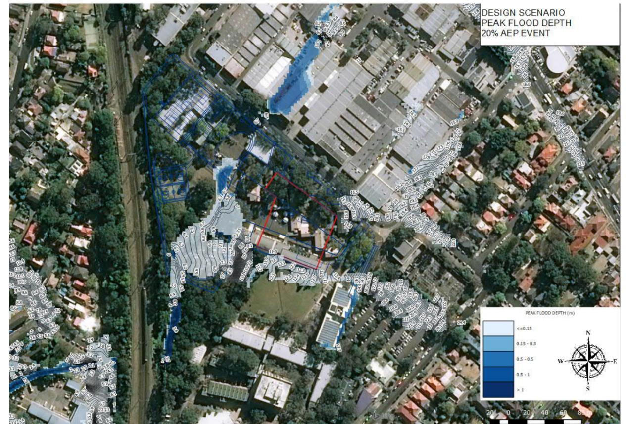
Figure 12. Overland flooding under post-development conditions for 20% AEP event
