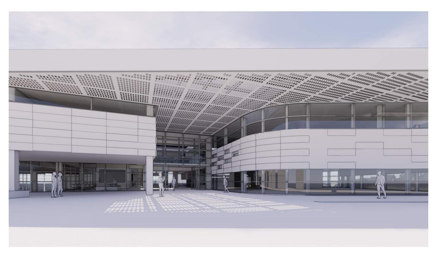
• THINNED FASCIA, FLATTENED SOFFIT AND TRANSPARENCY AT THE SEE STREET FACADE ADDITIONAL SKYLIGHT INTRODUCED AT SEE STREET ENTRY
