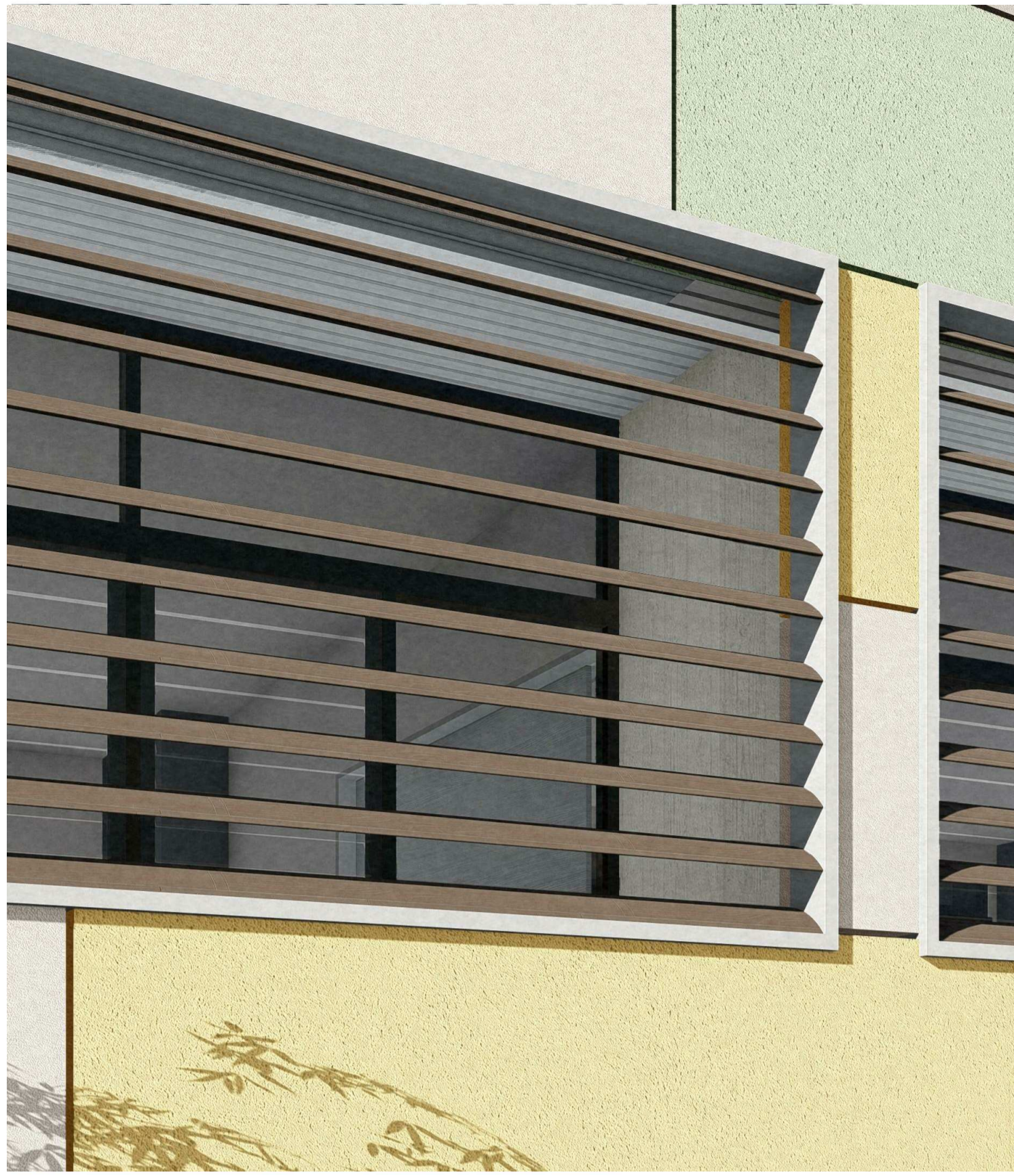
HORIZONTAL LOUVRES TO NORTH FACING HOMEBASES
