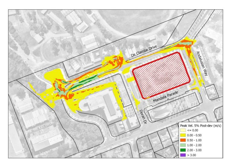
Figure 4.17 – Developed Scenario 5% AEP Flood Velocity
