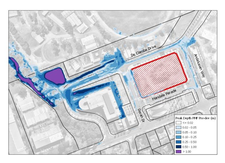
Figure 4.11 – Existing Scenario PMF Flood Depth
