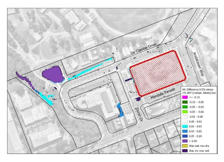
Figure 5.9 - Flood Level Difference - 0.5% AEP
