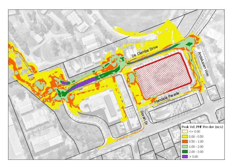
Figure 4.12 – Existing Scenario PMF Flood Velocity
