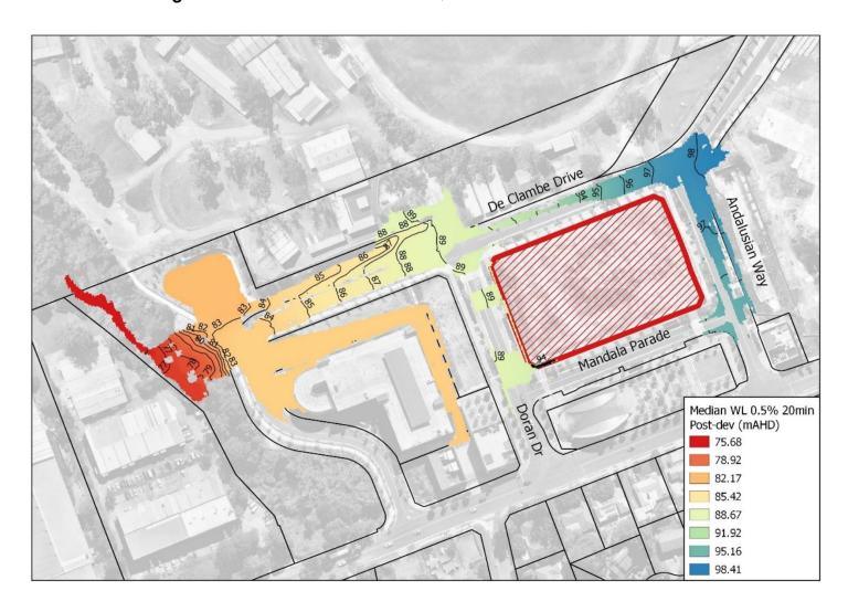
Figure 5.1 – Developed Scenario 0.5% AEP Flood Level
