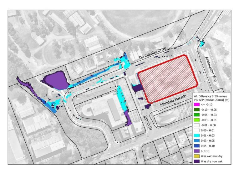
Figure 5.12 - Flood Level Difference - 0.2% AEP
