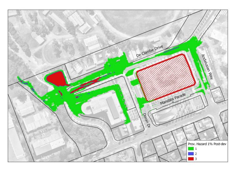
Figure 4.22 – Developed Scenario 1% AEP Flood Hazard (1 = Low 2 = Medium 3 = High)
