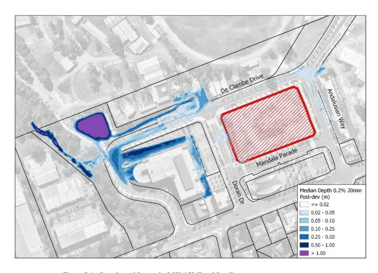
Figure 5.6 – Developed Scenario 0.2% AEP Flood Depth
