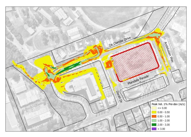
Figure 4.8 – Existing Scenario 1% AEP Flood Velocity
