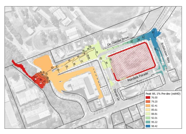
Figure 4.6 – Existing Scenario 1% AEP Flood Level
