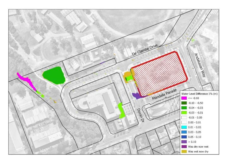
Figure 4.30 - Flood Level Difference - 1% AEP
