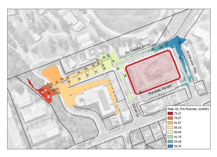
Figure 4.15 – Developed Scenario 5% AEP Flood Extent
