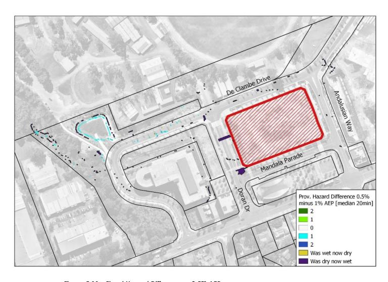
Figure 5.11 – Flood Hazard Difference – 0.5% AEP
