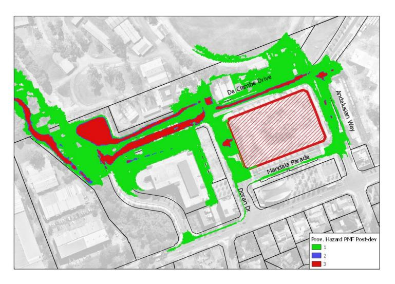
Figure 4.26 – Developed Scenario PMF Flood Hazard  $(1 = Low \ 2 = Medium \ 3 = High)$
