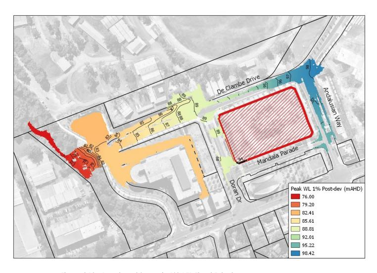
Figure 4.19 – Developed Scenario 1% AEP Flood Extent
