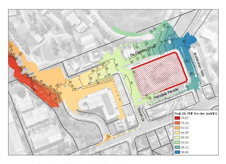
Figure 4.10 – Existing Scenario PMF Flood Level
