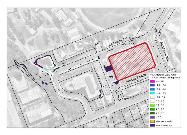
Figure 5.13 – Flood Velocity Difference – 0.2% AEP
