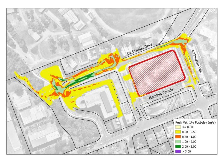
Figure 4.21 – Developed Scenario 1% AEP Flood Velocity
