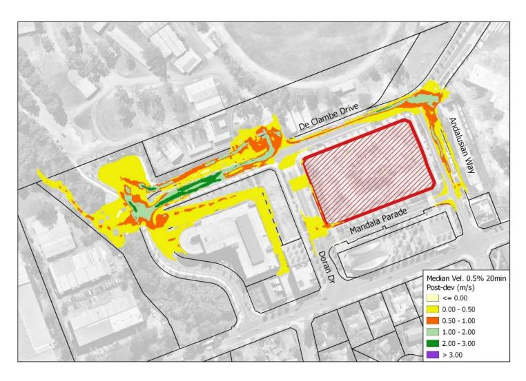
Figure 5.3 – Developed Scenario 0.5% AEP Flood Velocity
