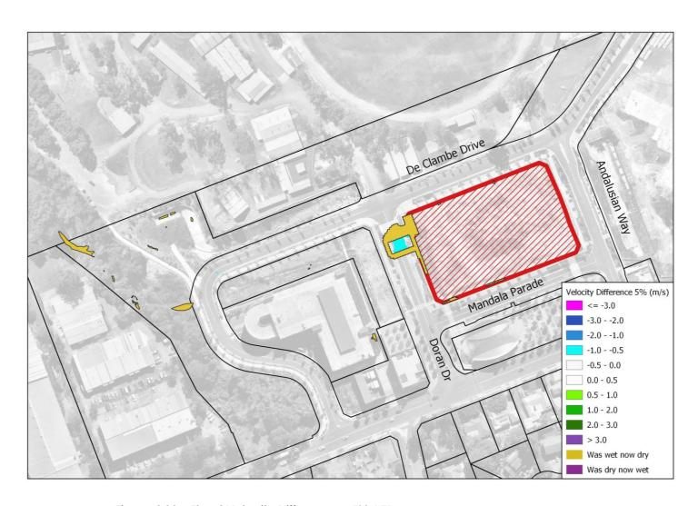
Figure 4.28 – Flood Velocity Difference – 5% AEP
