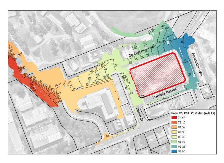
Figure 4.23 – Developed Scenario PMF Flood Level
