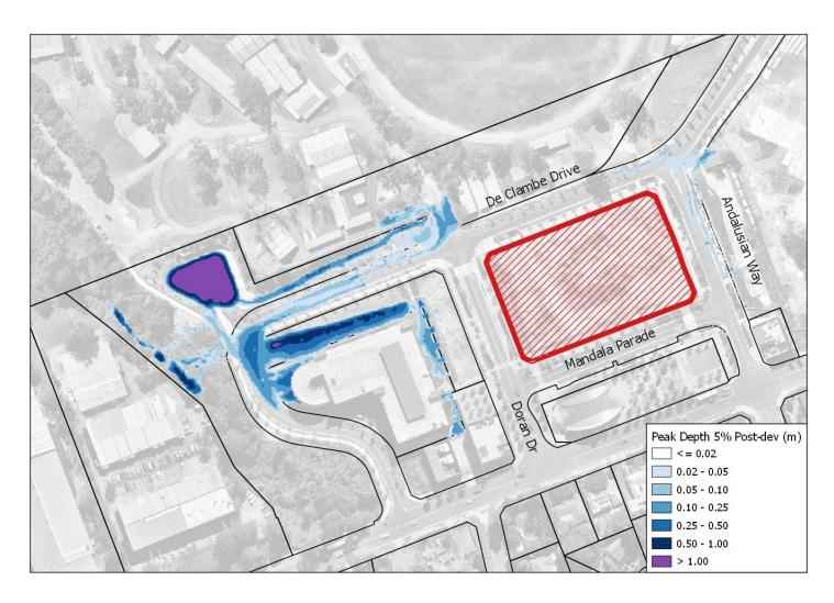
Figure 4.16 – Developed Scenario 5% AEP Flood Depth
