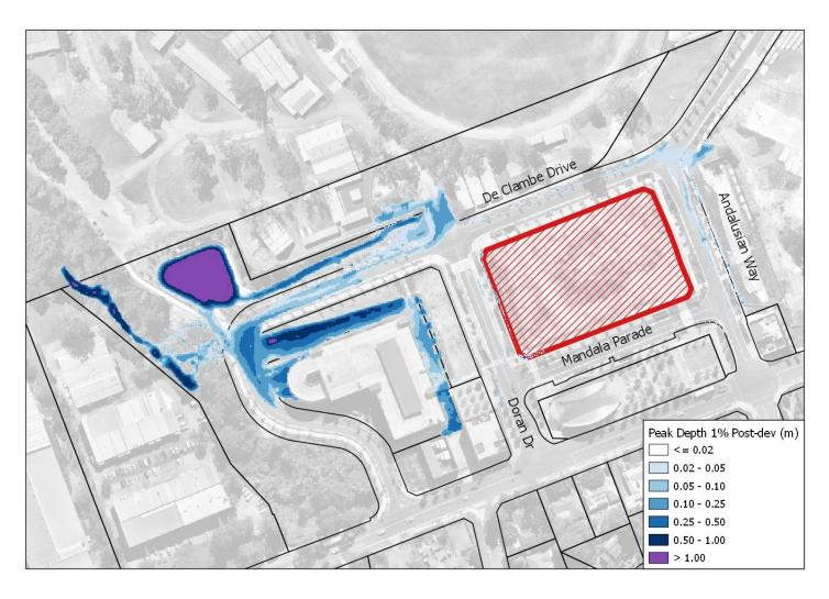
Figure 4.20 – Developed Scenario 1% AEP Flood Depth
