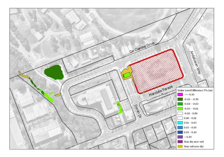
Figure 4.27 – Flood Level Difference – 5% AEP
