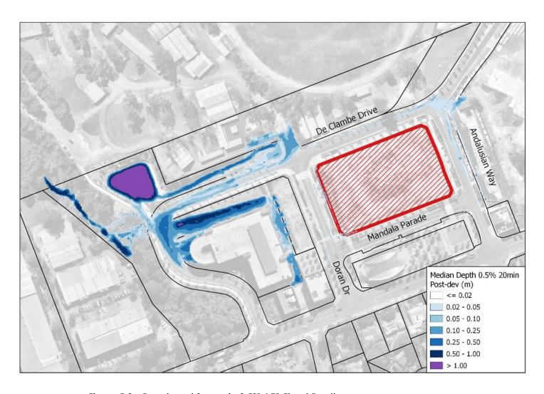
Figure 5.2 – Developed Scenario 0.5% AEP Flood Depth
