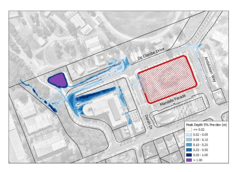
Figure 4.3 – Existing Scenario 5% AEP Flood Depth
