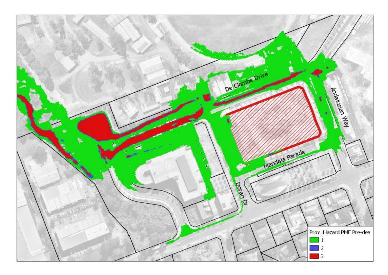
Figure 4.13 – Existing Scenario PMF Flood Hazard
