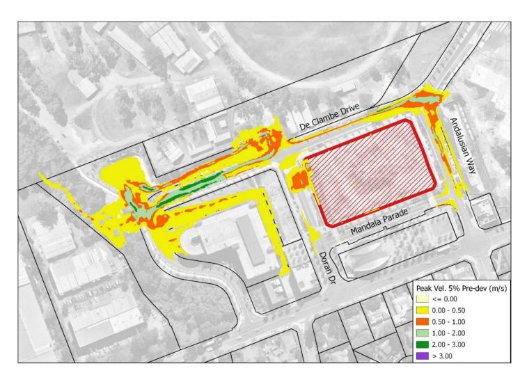
Figure 4.4 – Existing Scenario 5% AEP Flood Velocity
