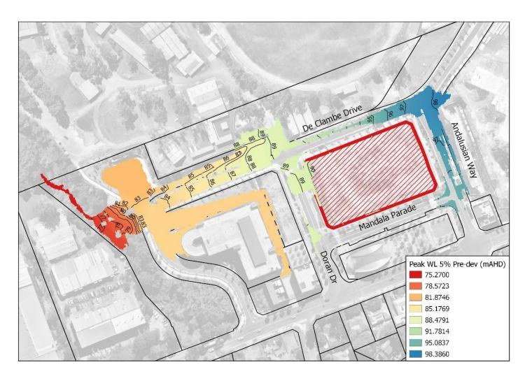
Figure 4.2 – Existing Scenario 5% AEP Flood Level
