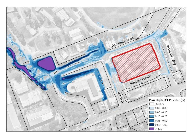
Figure 4.24 – Developed Scenario PMF Flood Depth
