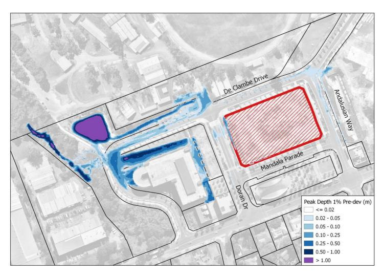
Figure 4.7 – Existing Scenario 1% AEP Flood Depth
