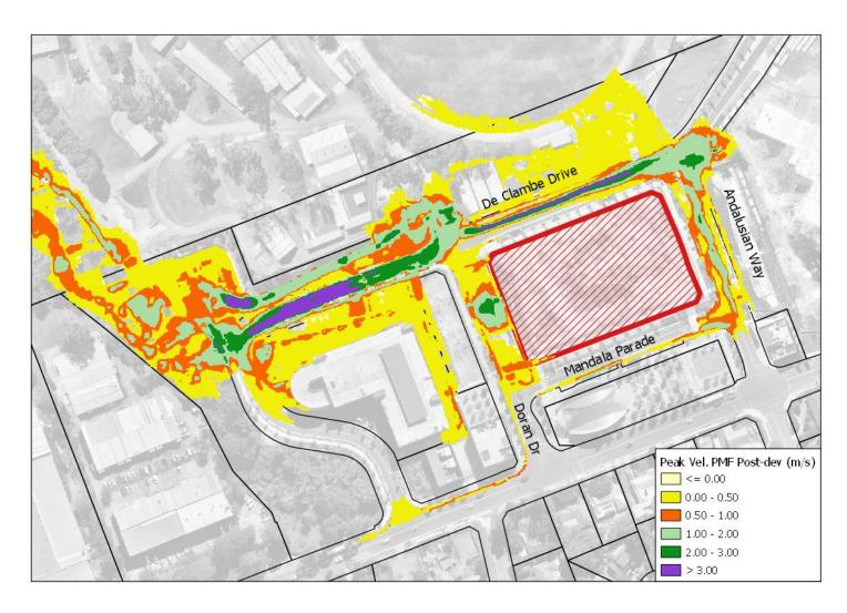
Figure 4.25 – Developed Scenario PMF Flood Velocity
