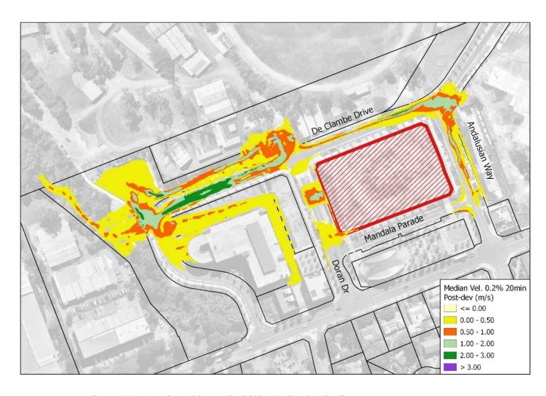
Figure 5.7 – Developed Scenario 0.2% AEP Flood Velocity
