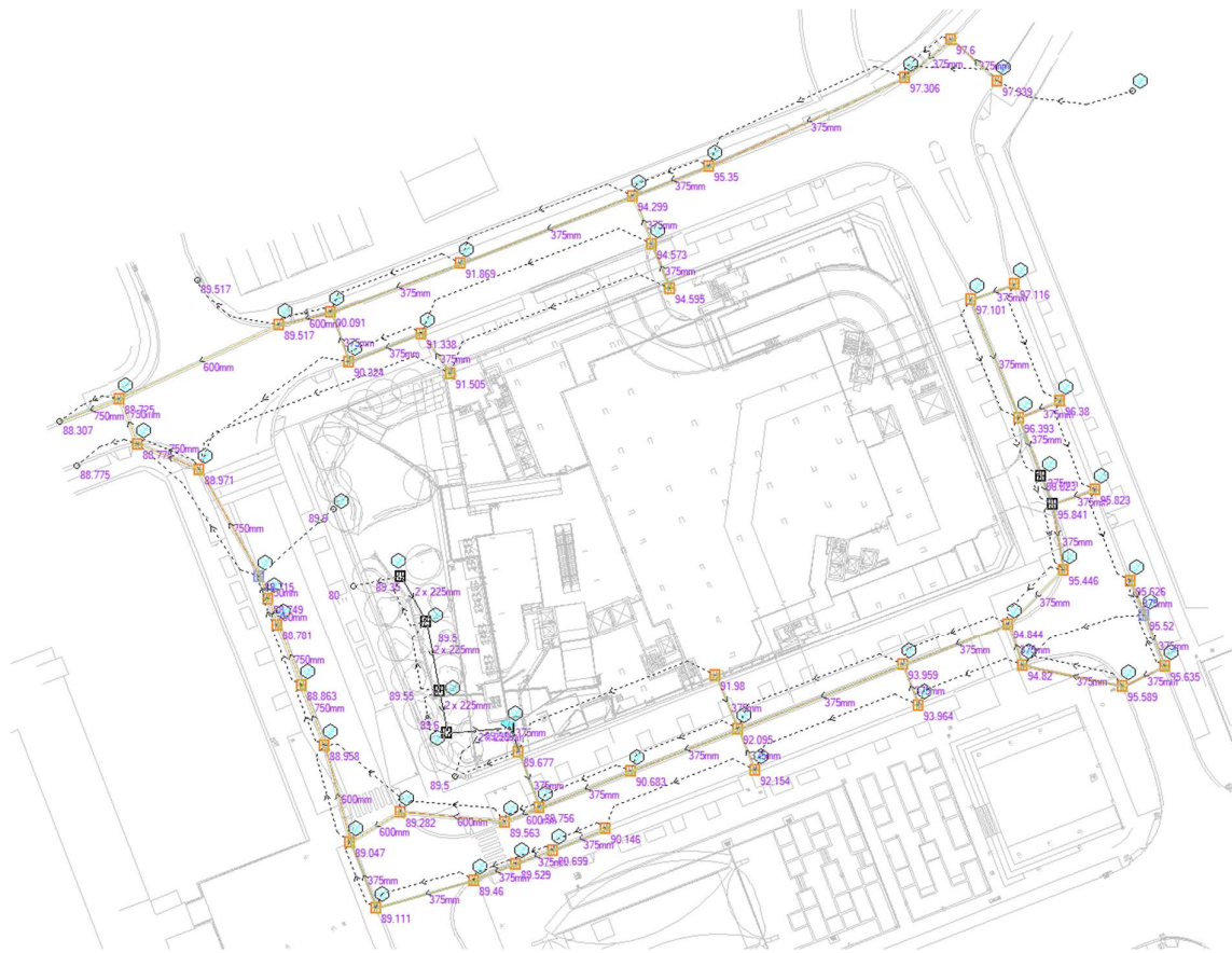
Figure 8 – Doran Drive DRAINS Model Schematic
