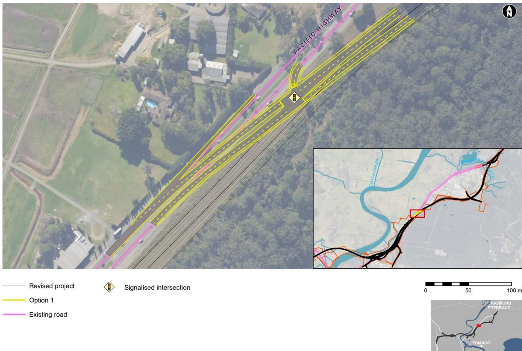
Figure 5-2 Proposed intersection layout of Option 1
