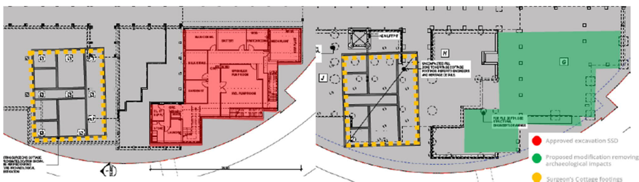
Figure 6 Comparison of excavation reduction between approved SSD (left) and proposed modification (right)
