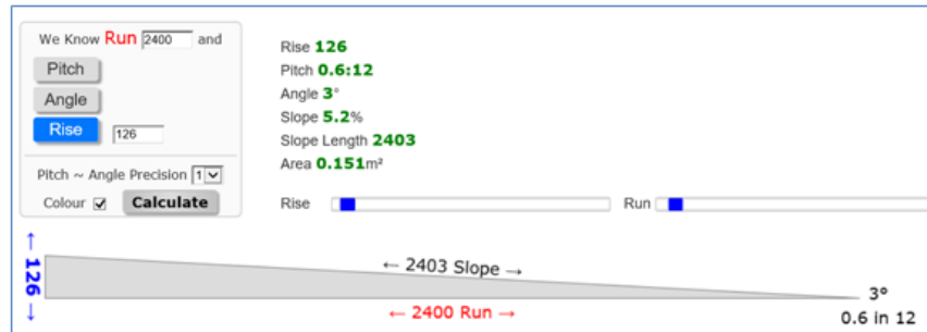
Figure 15 – 126mm over any 2.4 metres equates to an approximate a 3° degrees slope
