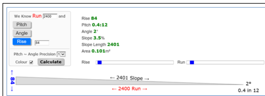
Figure 14 – 84mm over any 2.4 meters equates to an approximate a 2° degrees slope
