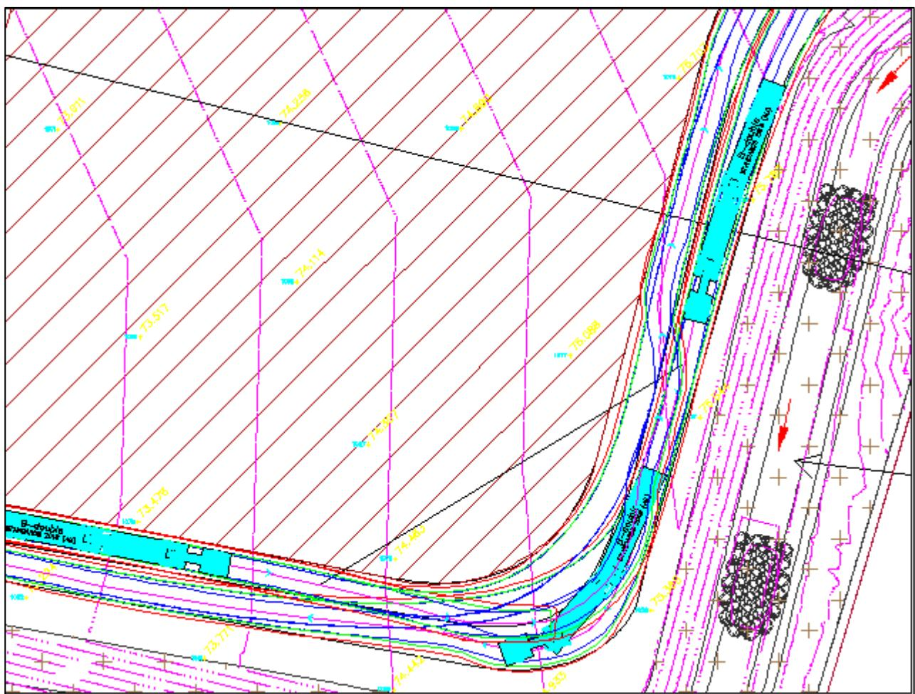
As shown above, two-way passing is not possible around the corner, while this is the case the above is a safe operation, as intervisibility is provided between passing areas.
