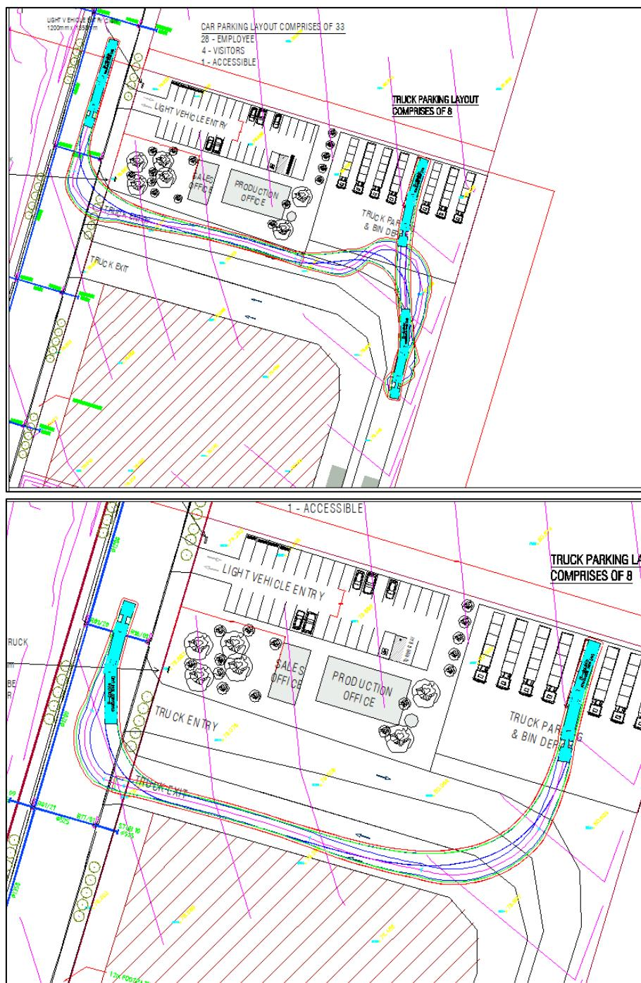
26m B-double into and out of truck parking area
