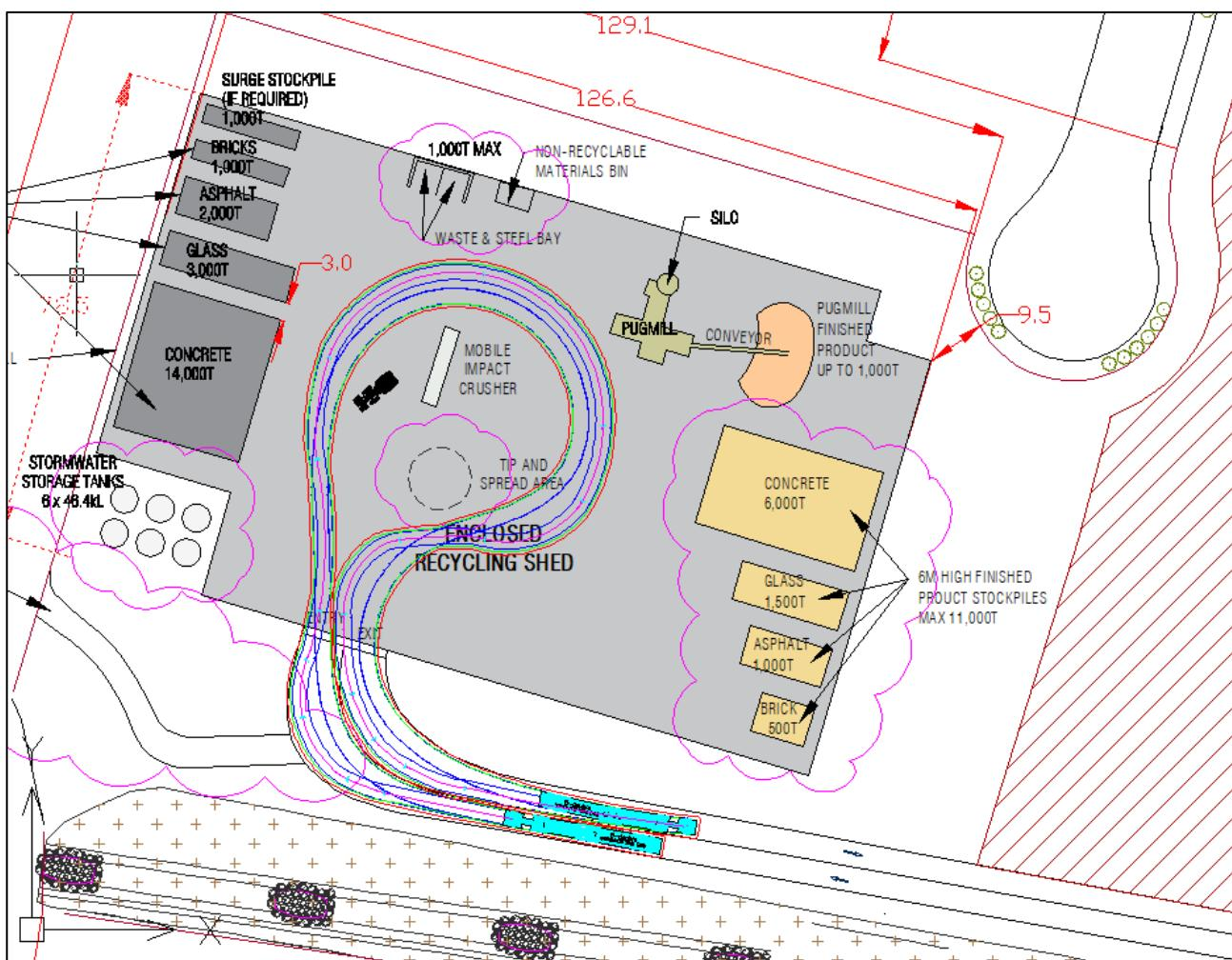
26m b-double turning around within the enclosed shed. Area shown above to be kept clear for circulation
