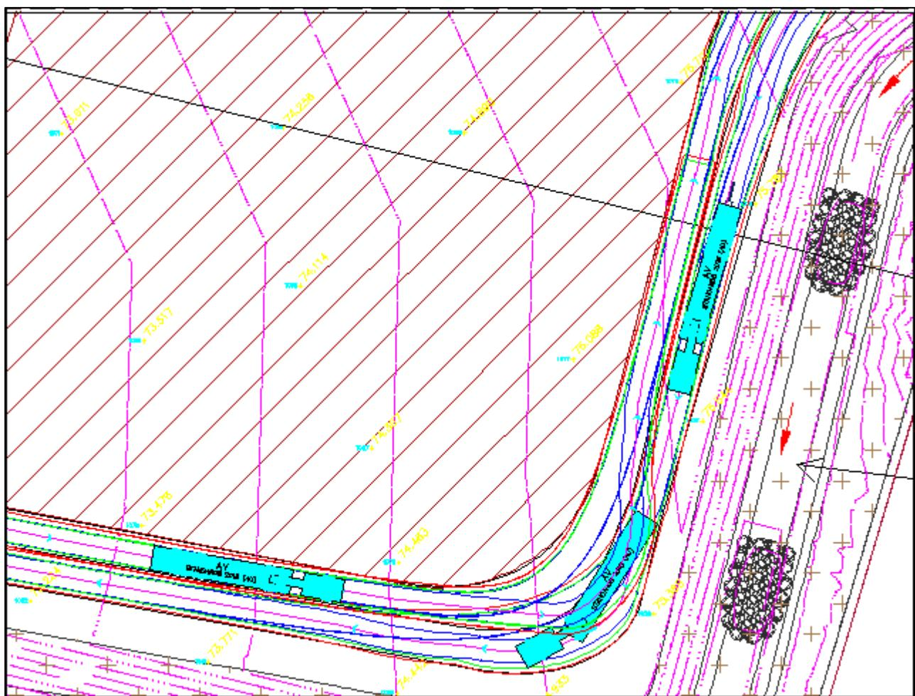
As shown above, two-way passing is not possible around the corner, while this is the case the above is a safe operation, as intervisibility is provided between passing areas.
