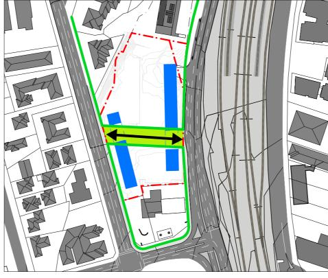
2. CREATE NEW THROUGH SITE LINK TO BREAK DOWN THE SCALE OF THE URBAN BLOCK AND INCREASE AREA CONNECTIVITY.
