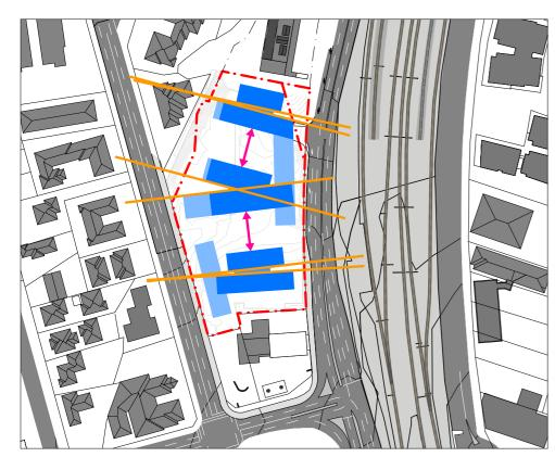
4. SHAPE AND ORIENT TALL BUILDINGS TO MAXIMISE SOLAR AMENITY, CROSS VENTILATION, AND ASPECT, AND TO **BREAK DOWN THE SCALE OF THE BUILDINGS**
