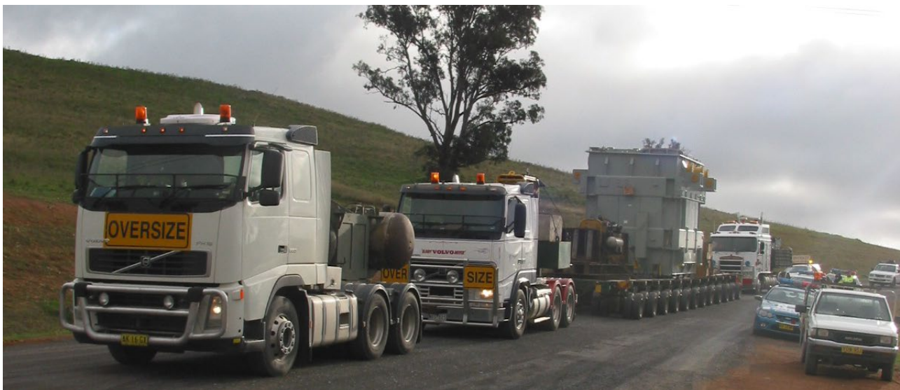
Photograph 4.1 Transformer delivery vehicle used for Bannaby substation
