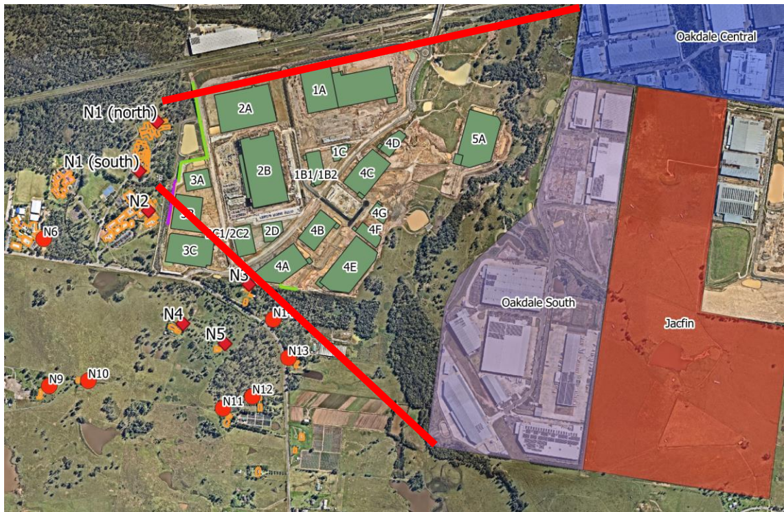
Figure 4-1 Screening of OWE between Receiver N1 and Industrial sites to the east
