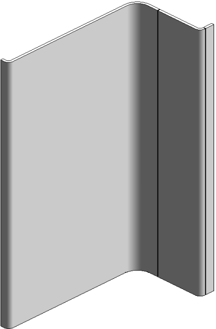
Proposed R5 Cladding, simple folded element, more adequate to suit the various steps and notches
