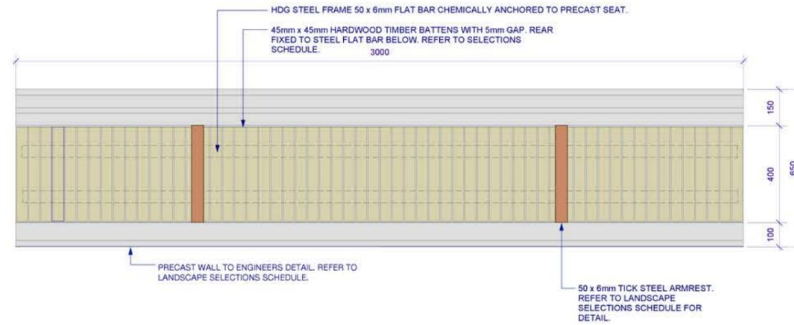
2 WALL TYPE 1 - PRECAST CONCRETE WALL WITH INTEGRATED TIMBER BENCH
