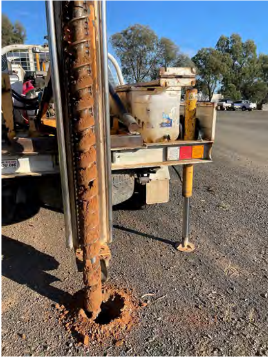
Figure 9. SP5 borehole displaying dry, natural soil
