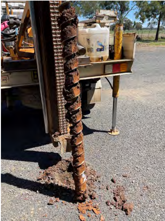
Figure 33. SP29 borehole displaying dry, natural soil beneath 200mm of road base/fill
