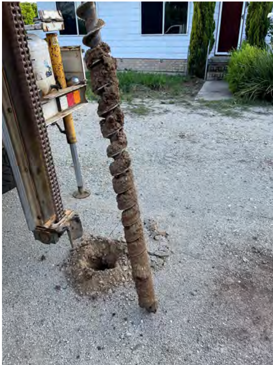
Figure 5. SP1 borehole displaying dry, natural soil
