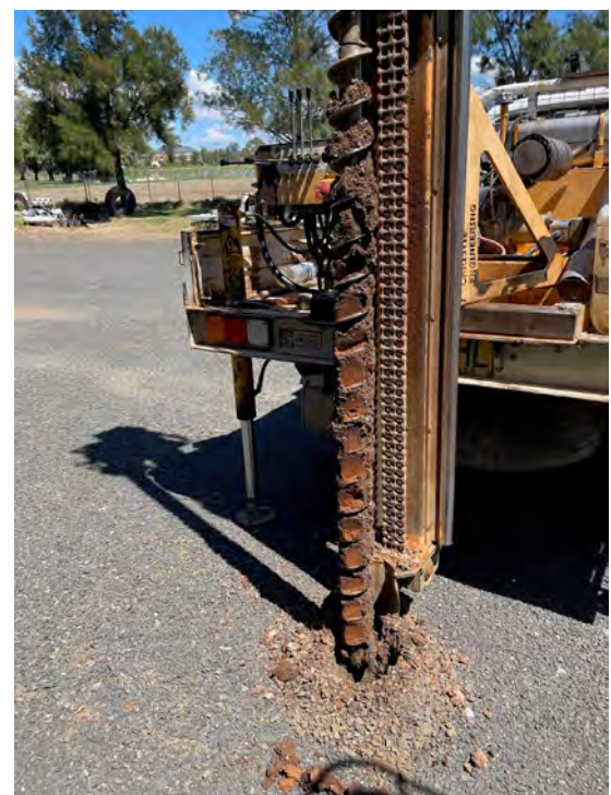
Figure 32. SP28 borehole displaying dry, natural soil beneath 100mm of road base/fill
