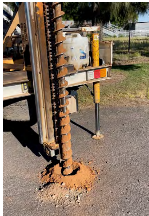
Figure 12. SP8 borehole displaying dry, natural soil beneath 100mm of road base/fill
