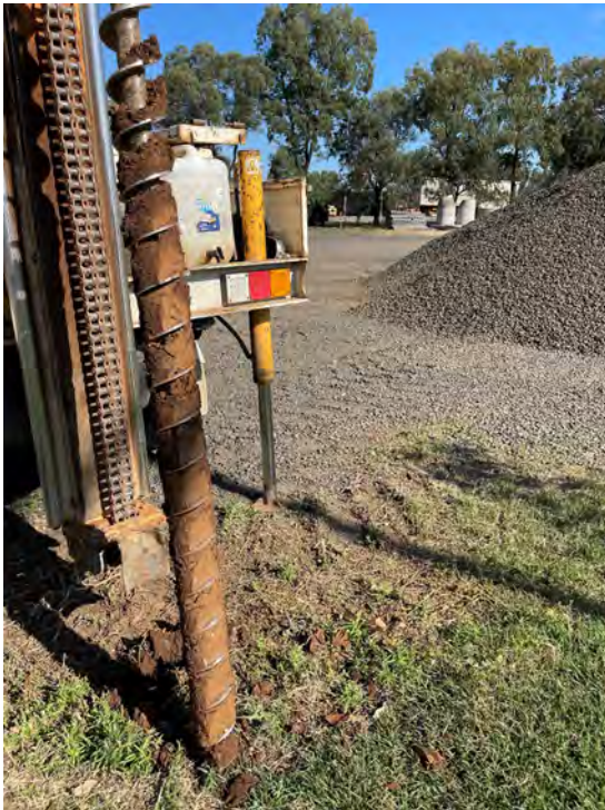
Figure 17. SP13 borehole displaying dry, natural soil beneath 400mm of road base/fill
