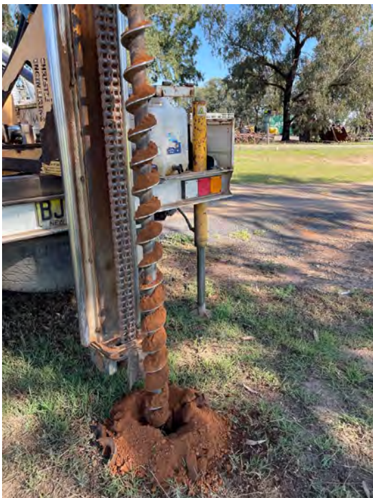
Figure 19. SP15 borehole displaying dry, natural soil
