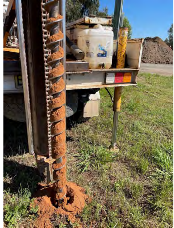
Figure 26. SP22 borehole displaying dry, natural soil beneath 200mm of road base/fill
