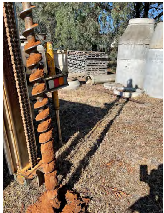
Figure 20. SP16 borehole displaying dry, natural soil
