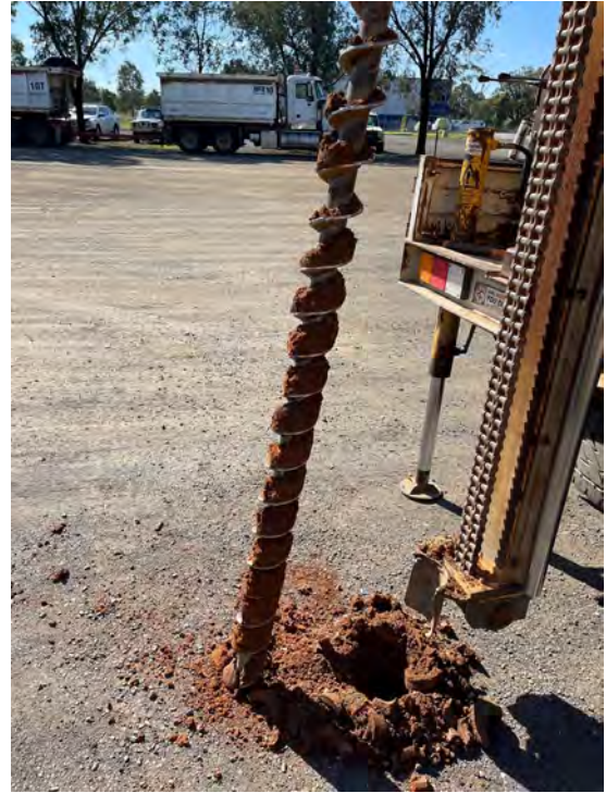
Figure 22. SP18 borehole displaying dry, natural soil beneath 300mm of road base/fill
