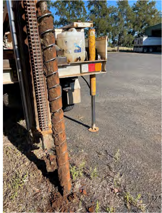
Figure 14. SP10 borehole displaying dry, natural soil beneath 150mm of road base/fill
