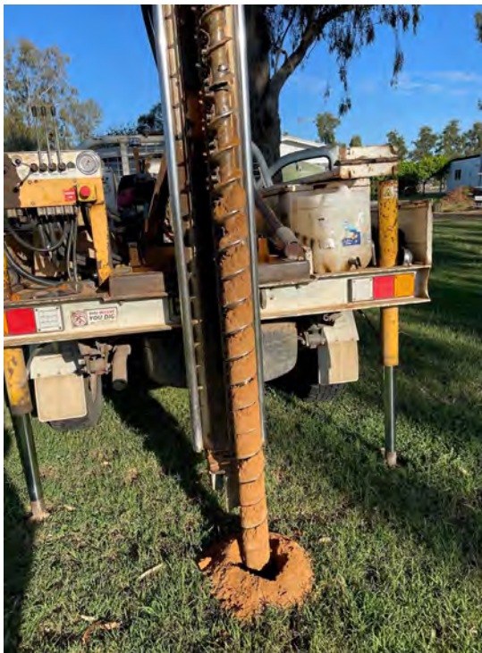
Figure 7. SP3 borehole displaying dry, natural soil
