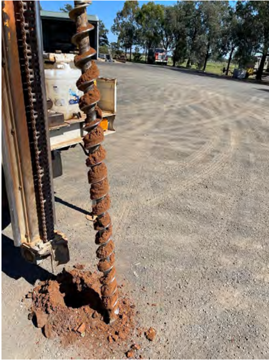
Figure 25. SP21 borehole displaying dry, natural soil beneath 400mm of road base/fill
