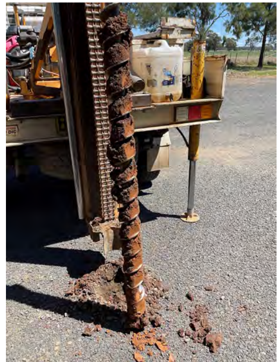
Figure 28. SP24 borehole displaying dry, natural soil
