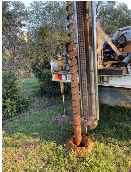
Figure 6. SP2 borehole displaying dry, natural soil
