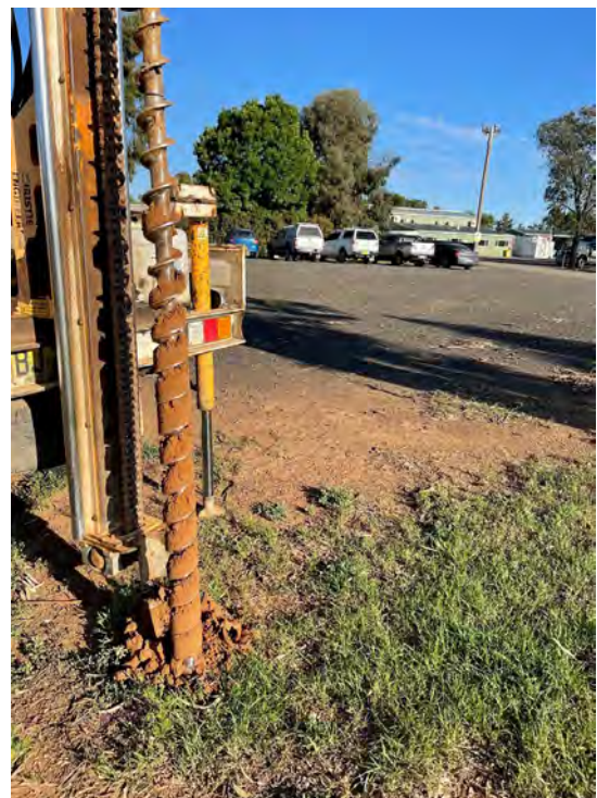
Figure 8. SP4 borehole displaying dry, natural soil
