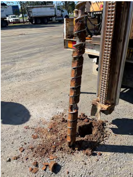
Figure 23. SP19 borehole displaying dry, natural soil beneath 400mm of road base/fill
