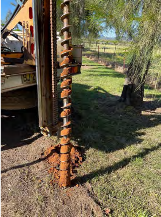
Figure 13. SP9 borehole displaying dry, natural soil beneath 100mm of road base/fill
