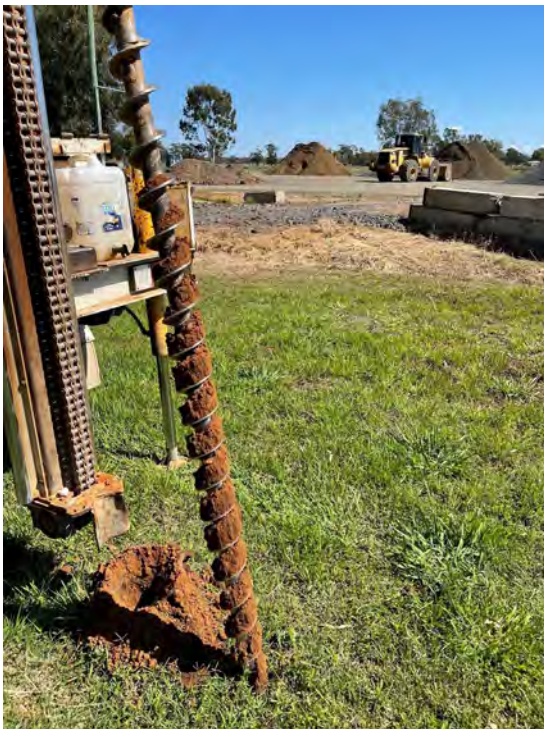
Figure 27. SP23 borehole displaying dry, natural soil
