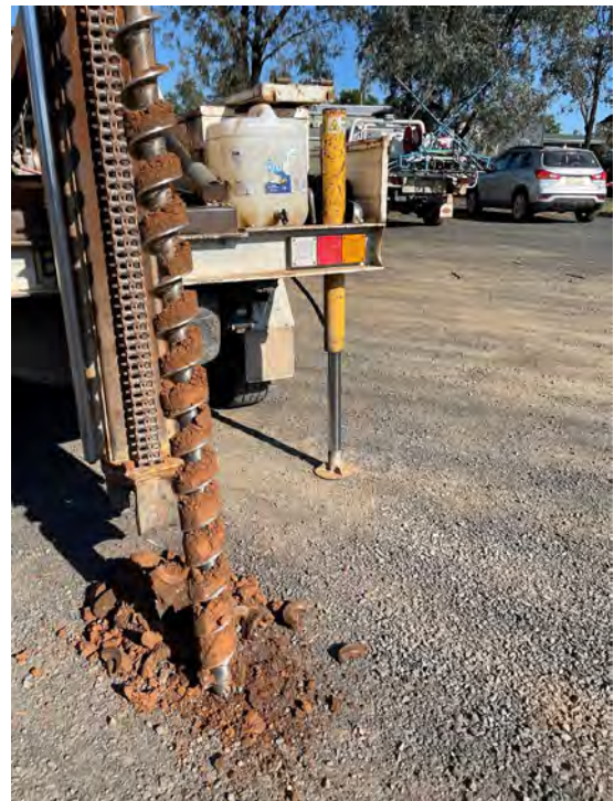
Figure 16. SP12 borehole displaying dry, natural soil beneath 100mm of road base/fill
