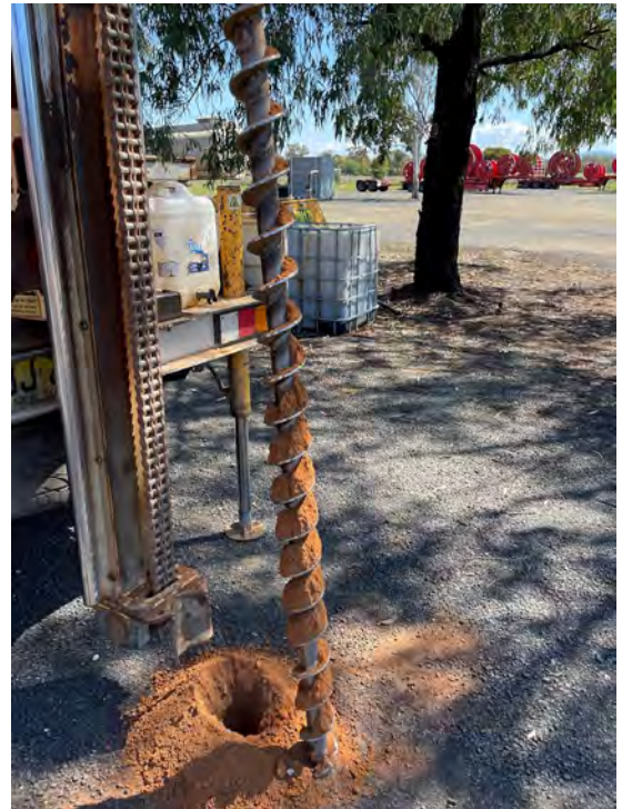
Figure 30. SP26 borehole displaying dry, natural soil beneath 300mm of road base/fill
