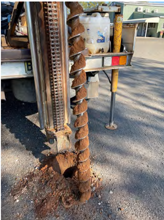
Figure 15. SP11 borehole displaying dry, natural soil beneath 300mm of road base/fill
