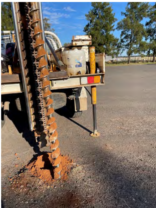
Figure 11. SP7 borehole displaying dry, natural soil beneath 150mm of road base/fill
