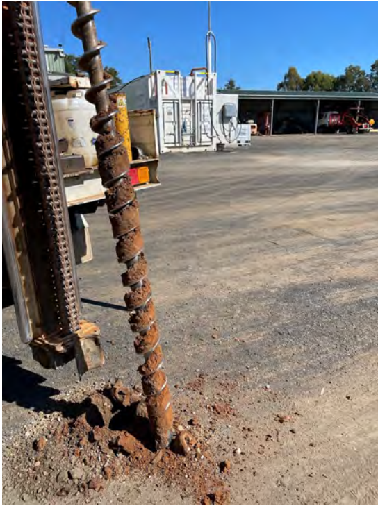
Figure 21. SP17 borehole displaying dry, natural soil beneath 400mm of road base/fill
