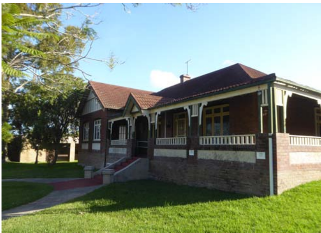
Figure 3.9 The house is a reasonably mainstream Federation Bungalow, originally built as a four room dwelling with verandah around three sides. The large side gable is located over a large room that replaced the southern side verandah of the house several years after it was first built.
