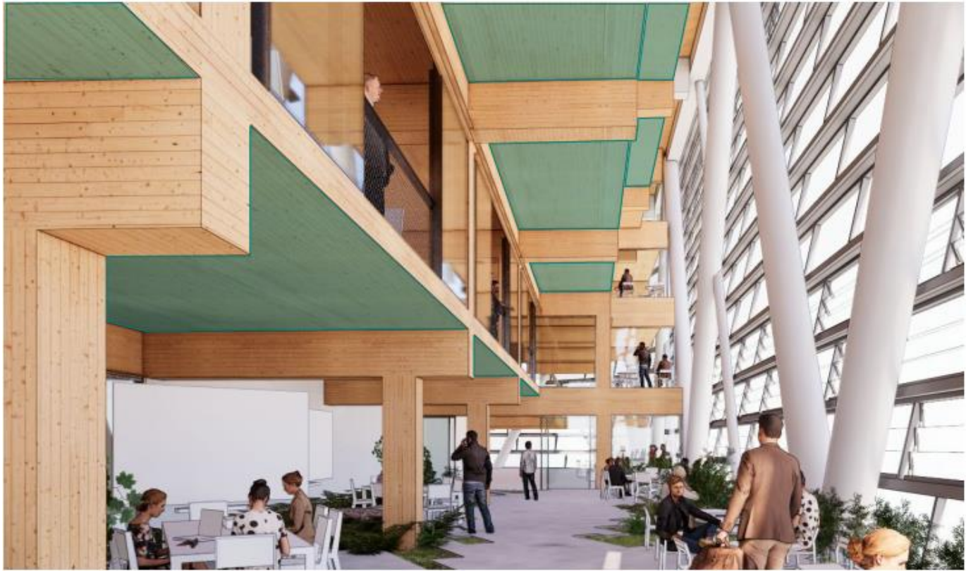
Figure 15: Proposed acoustically absorptive panelling to the outdoor habitats – shaded in green
