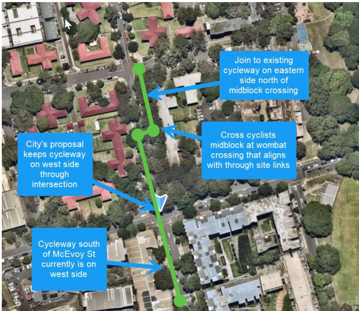
Figure 4 Transition of cycleway through the intersection
