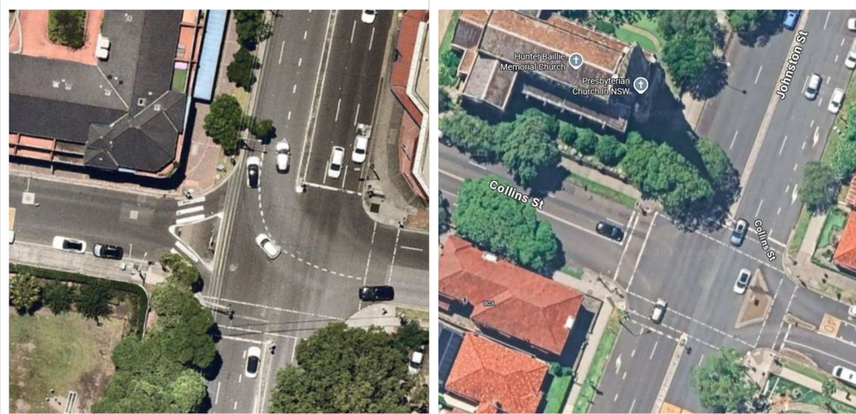
Figure 1. Figure 7 Examples of medians to control traffic movements in Sydney intersections : (a) Morwick / The Boulevard, Strathfield : Western approach to signals priority controlled with zebra crossing, plus restricts through movements in a signalised intersection using physical median (b) Johnson / Collins, Annadale : Restricts through movements in a signalised intersection using physical median
