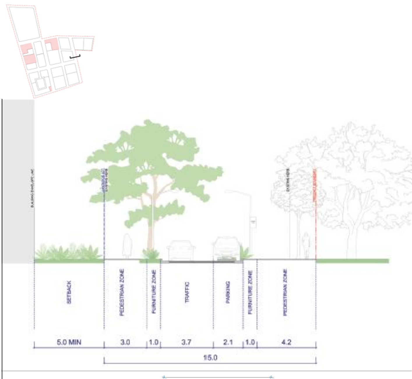
Figure 8(c): STREET CROSS SECTION – Pitt Street extension
