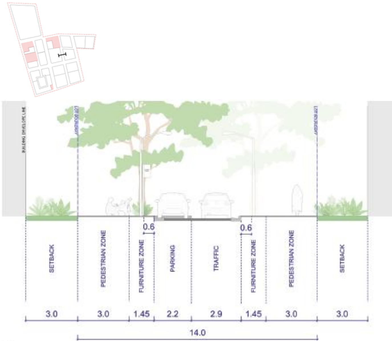
Figure 8(e): STREET CROSS SECTION – West Street
