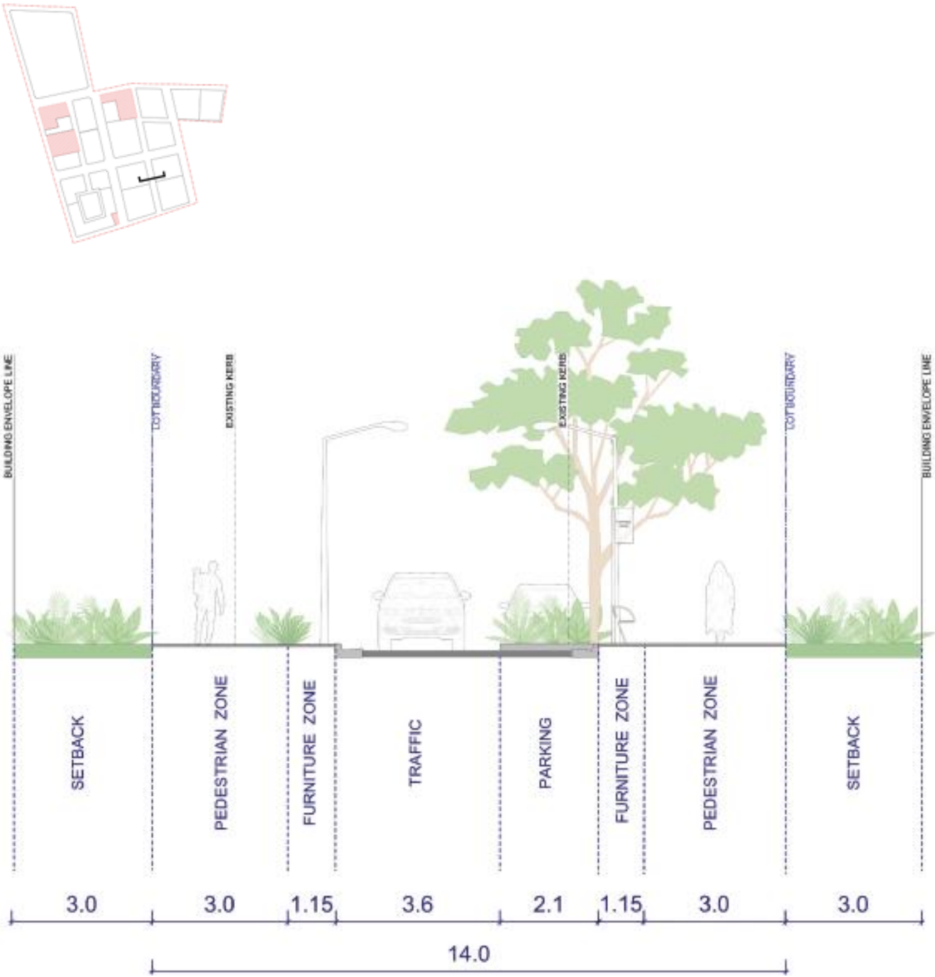
Figure 8(f): STREET CROSS SECTION – Mead Street
