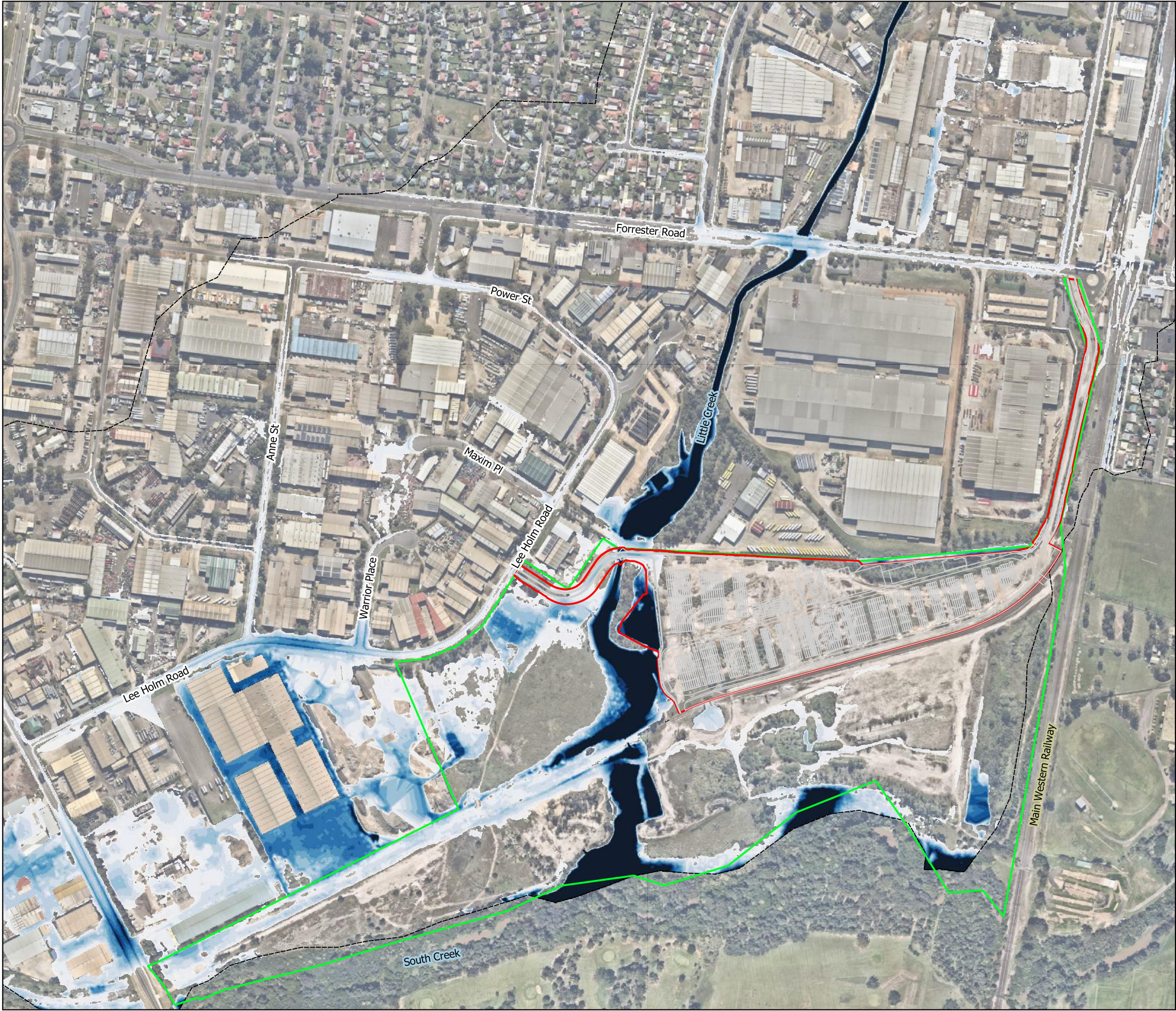
ST MARYS INTERMODAL Figure C6 - Post-Development Flood Depths 5% AEP event
