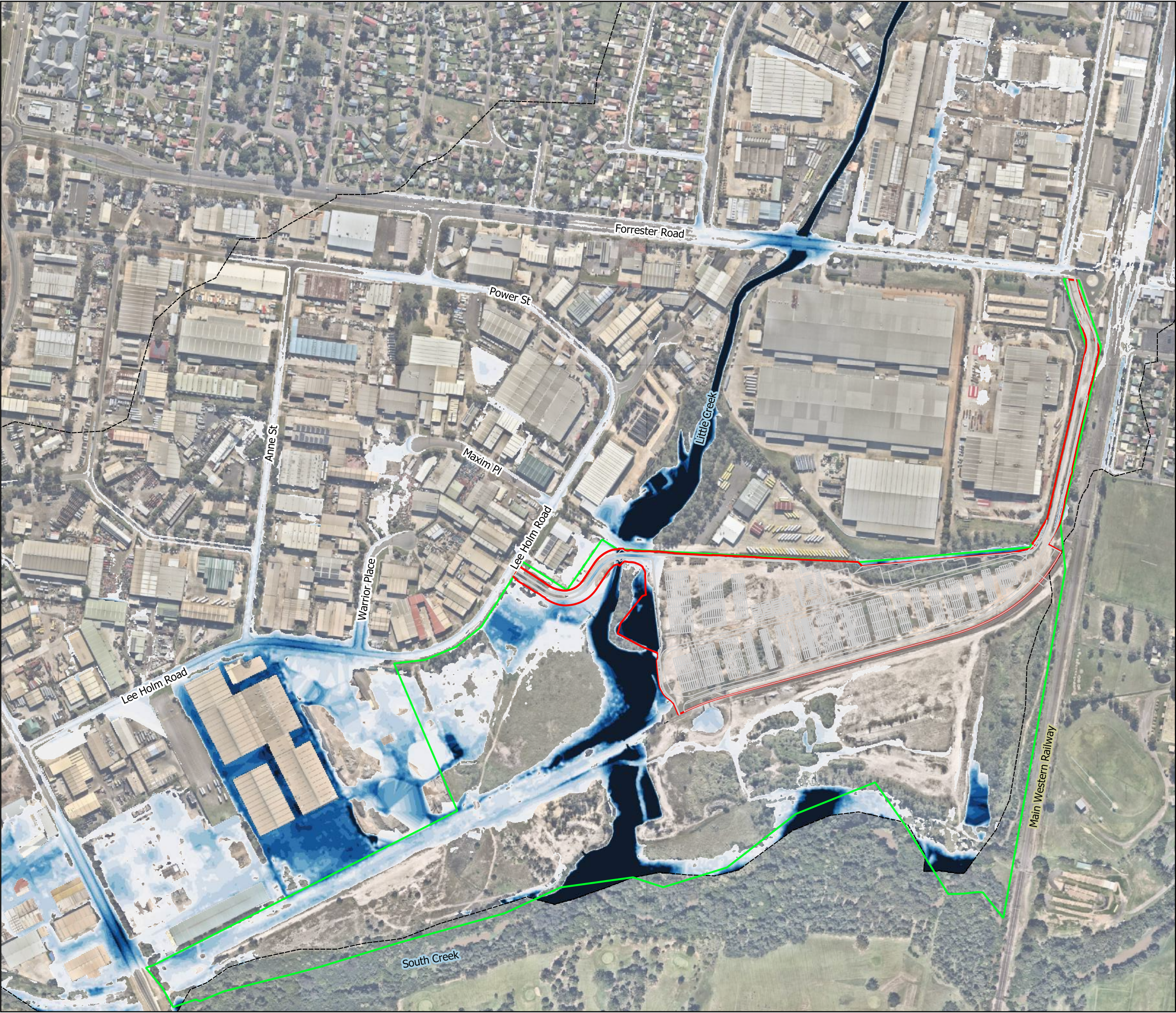
ST MARYS INTERMODAL Figure C7 - Post-Development Flood Depths 1% AEP event
