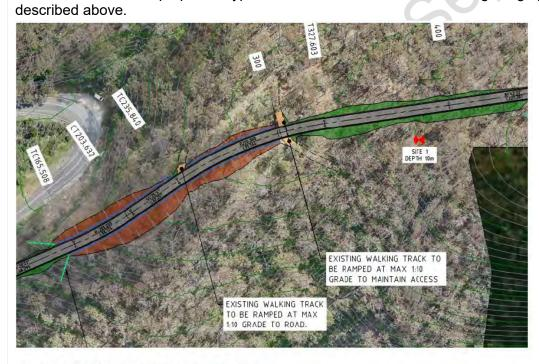
Figure 3-3: Existing pedestrian access track tie ins
