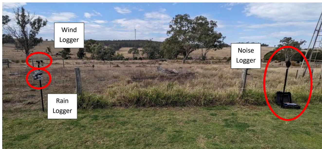
Figure 2: Typical Monitoring Location Setup
