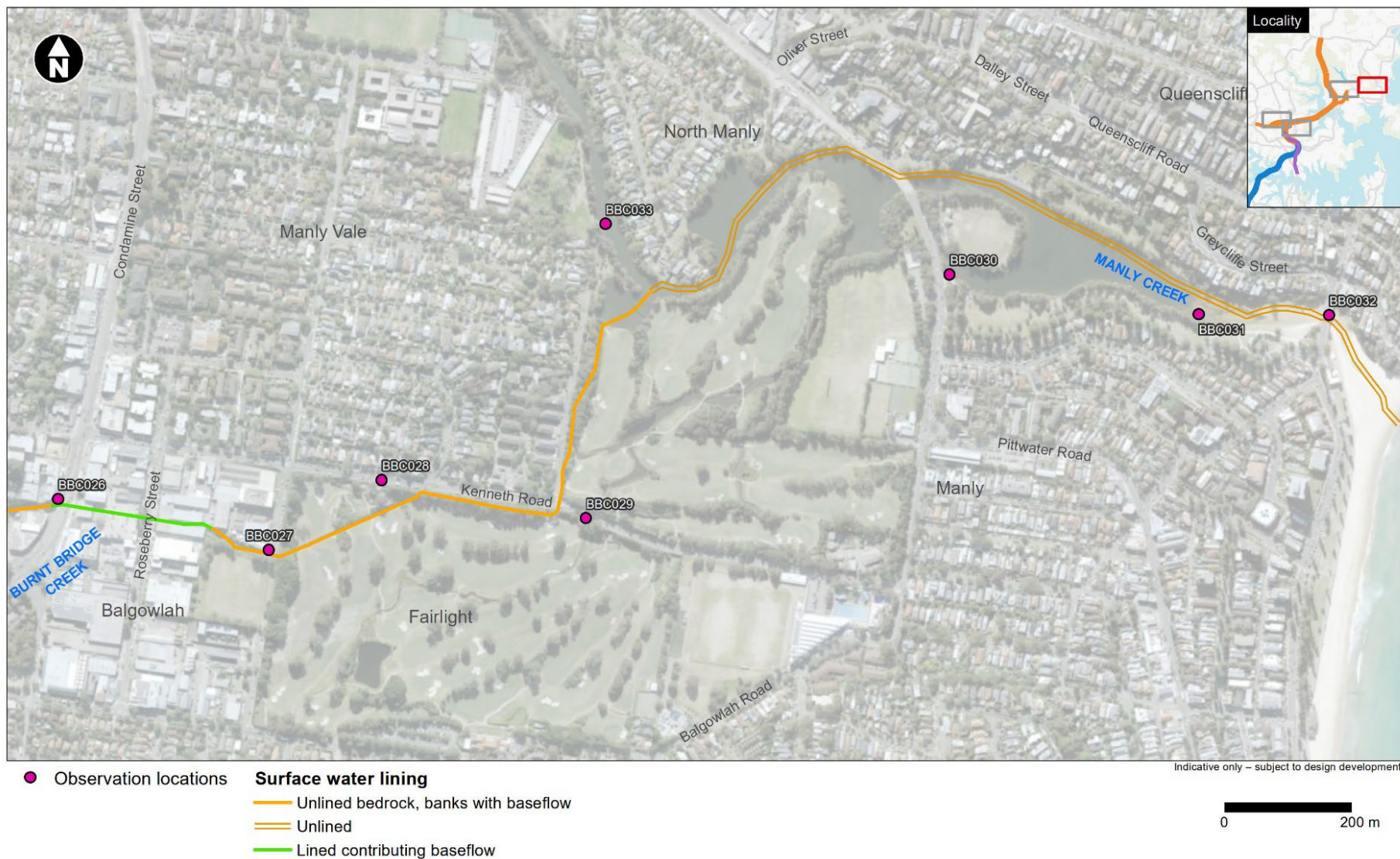
Figure 7. Waterway lining type - lower reach of Burnt Bridge Creek
