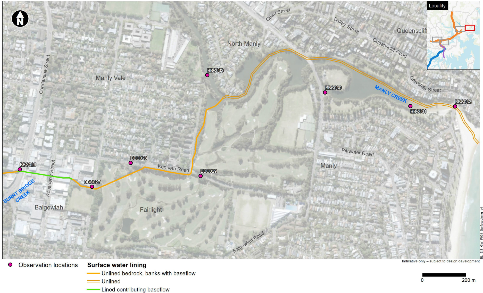
Figure 3-13 Burnt Bridge Creek surface lining (downstream extent) (Source: Jacobs, 2021)
