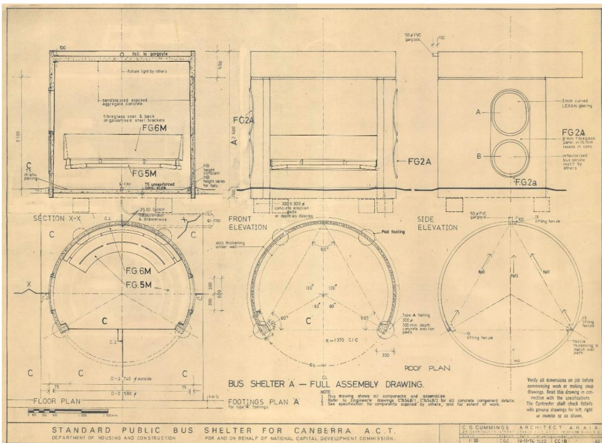
Figure 2-2 Standard Public Bus Shelter for Canberra ACT, Plans for the Series I concrete bus shelter (Archives ACT CT-CC1B)
