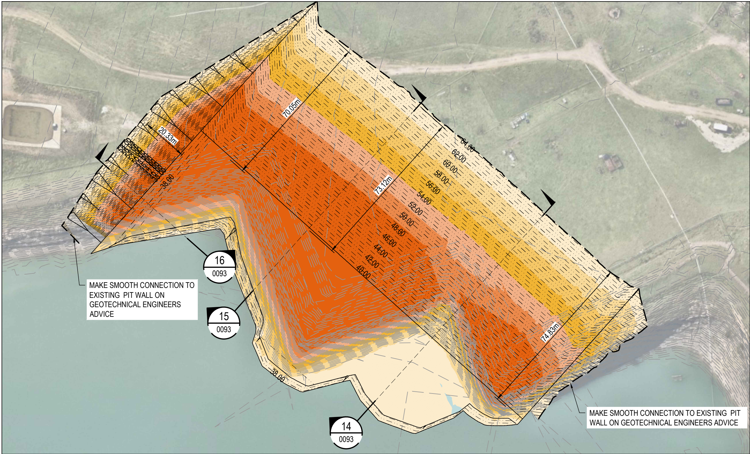
PIT 1 - NORTHERN EXCAVATION DEPTH RANGE
