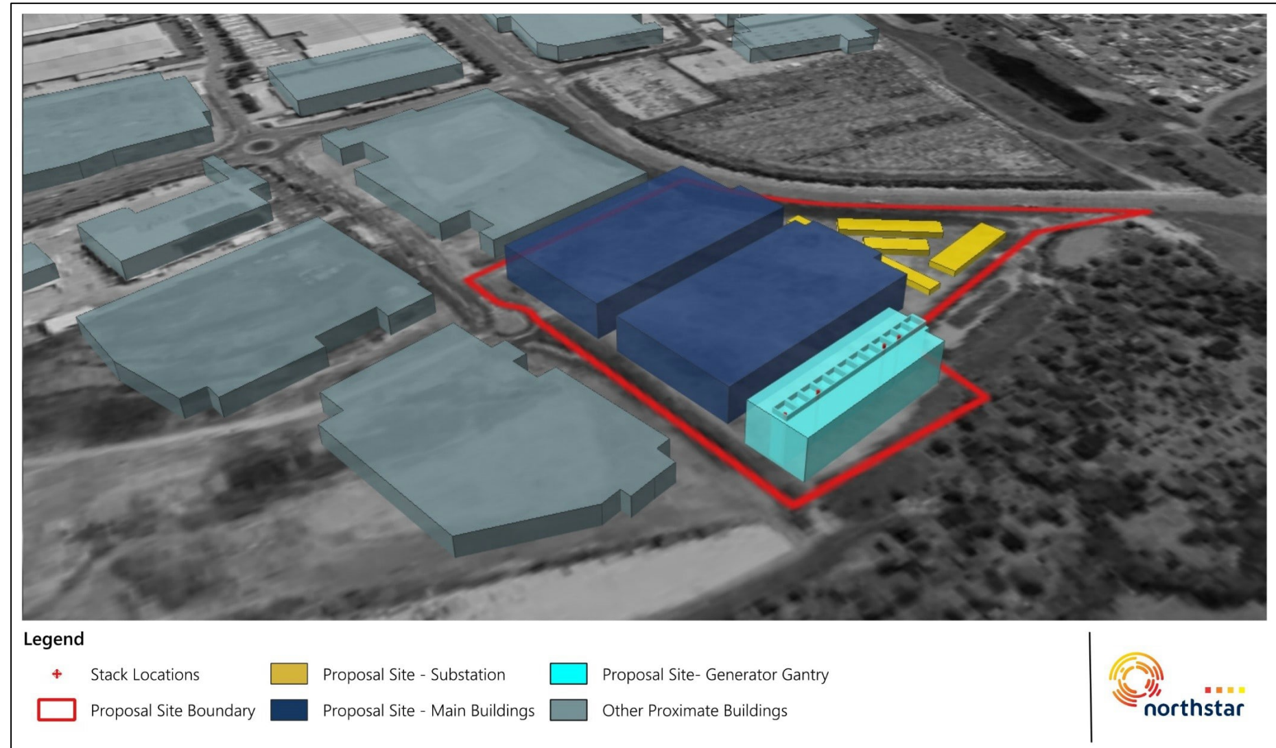
Figure 9 Buildings and discharge points considered in dispersion modelling (Scenario 2)
