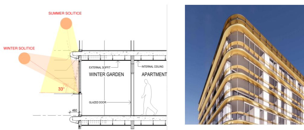
Figure 2: Shading Device Design; Source: AJC/JHA
