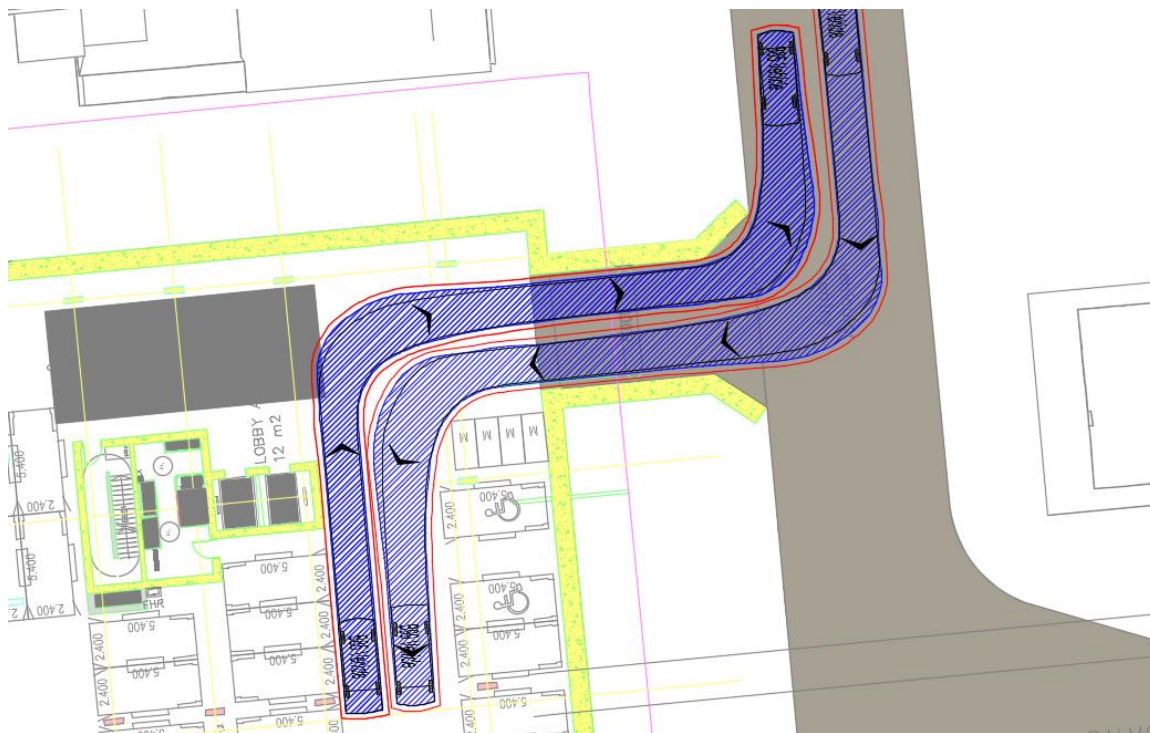
Figure 11 Swept path analysis – access for passenger vehicles
