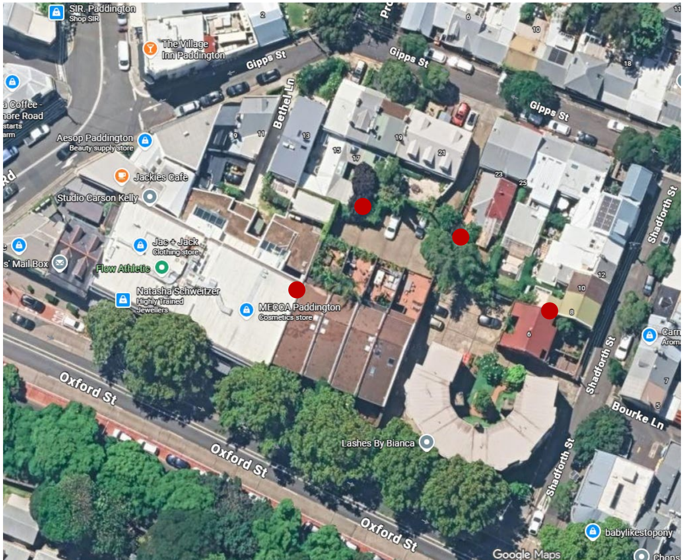
Figure 2 Location of vibration monitoring points ● Vibration Monitor Location
