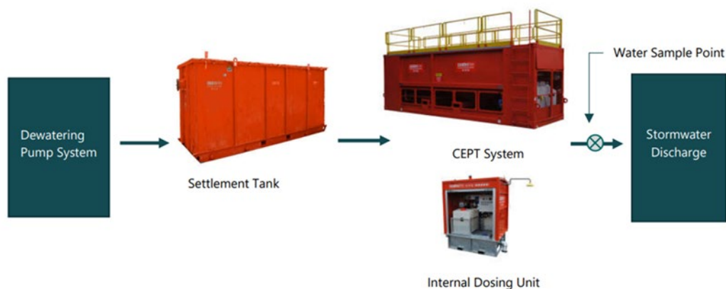
Figure 6: Indicative possible treatment system where analyte values exceed Council, ANZG or NEPM threshold values
