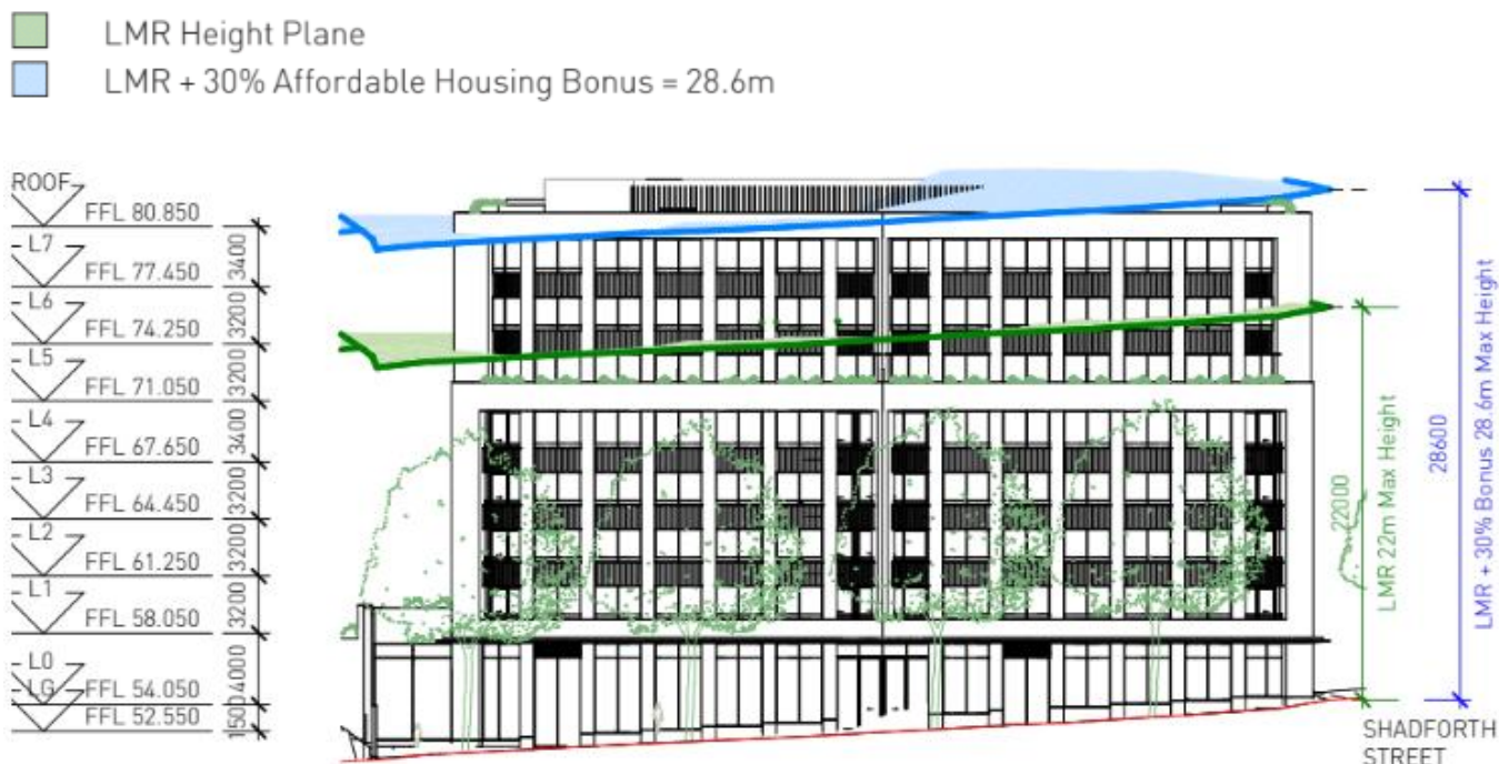
Figure 29 Proposed Southern Elevation showing LMR height plane (22m, green) and LMR height plane (combined with affordable housing bonus) (28.6m blue)
