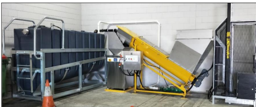
Figure 6 – Example Macerator (left) and food organics trolley (right).
