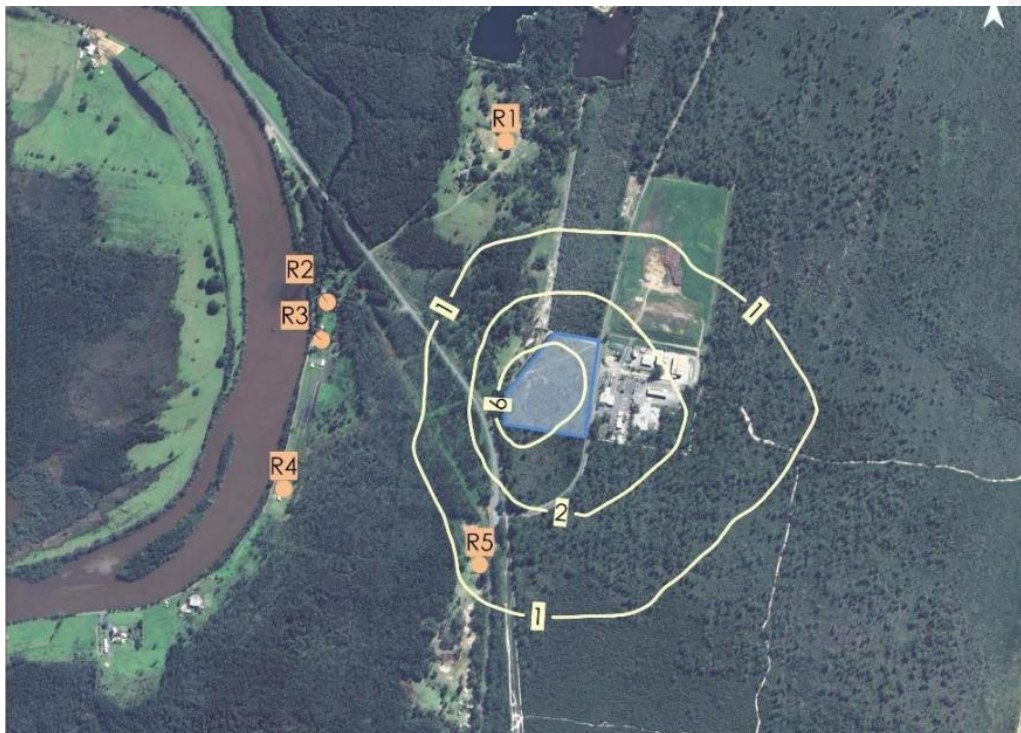
Figure 24: 99 th percentile nose-response ground level hour concentrations
