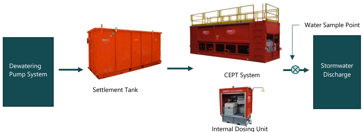
Figure 12-1 Water Treatment Plant Process Diagram
