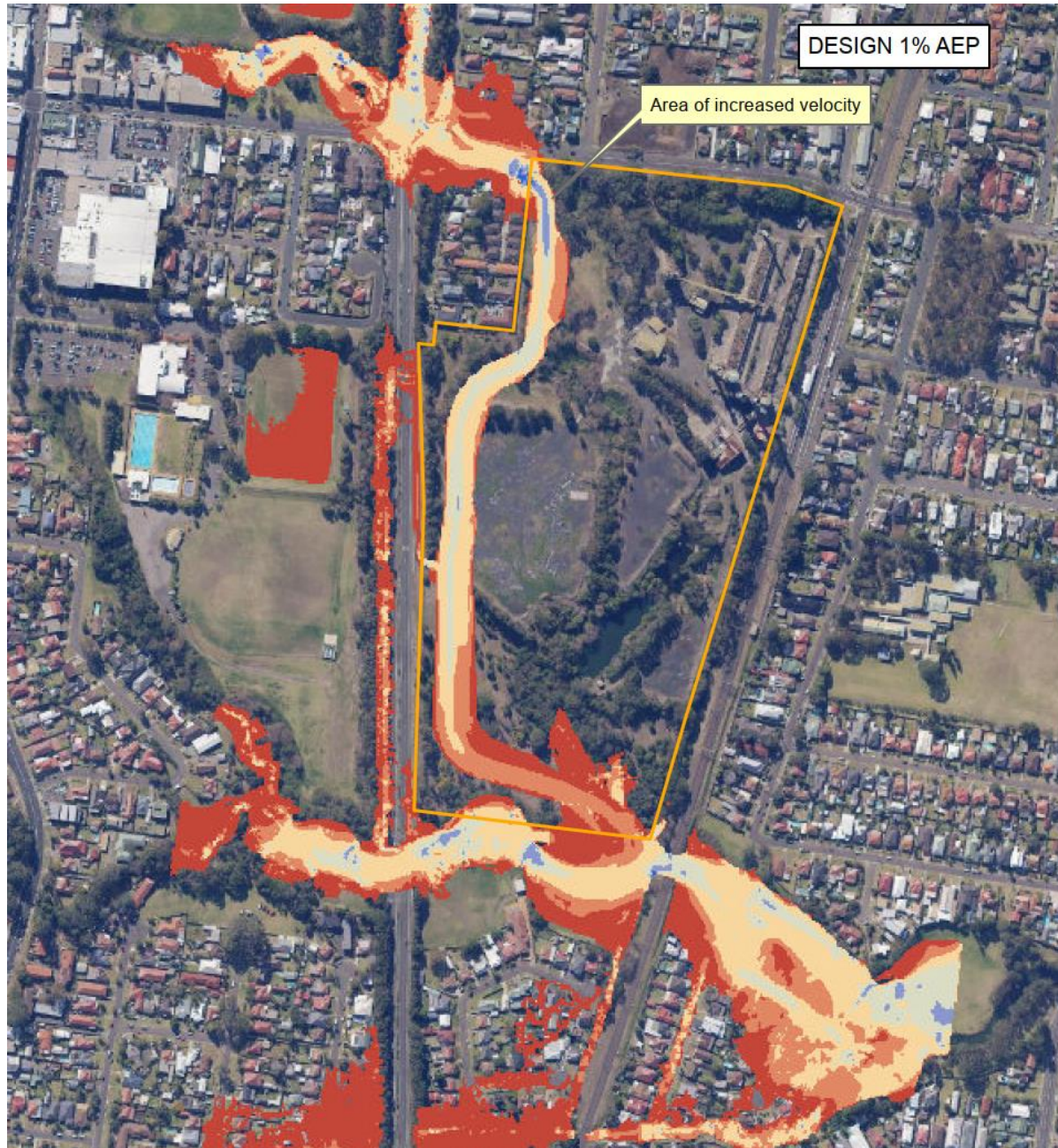
Figure 9: Proposed Design Velocities 1% AEP (Geomorphology Assessment, ICC Redevelopment)
