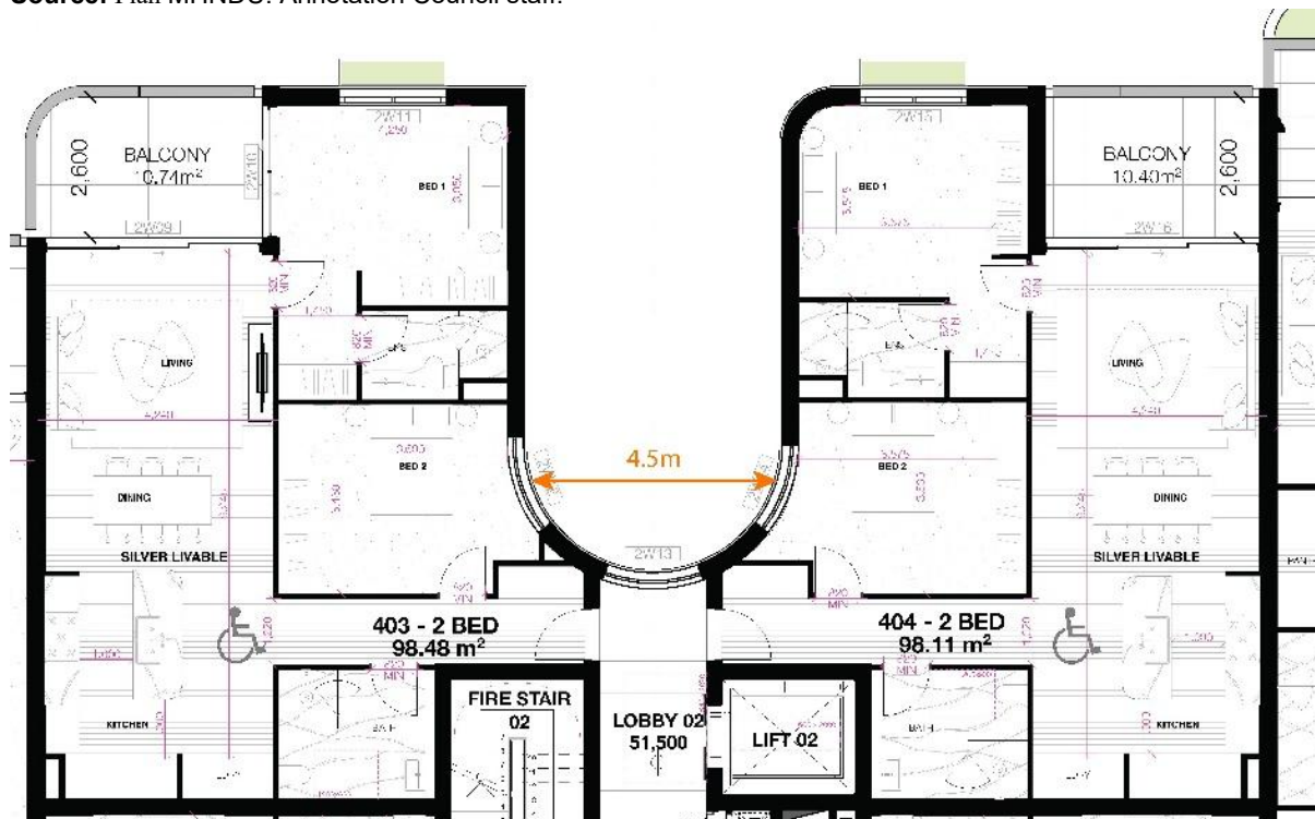
Figure 6: Level 02 plan illustrating direct overlooking between Bedroom 2. Source: Plan MHNDU. Annotation Council staff.
