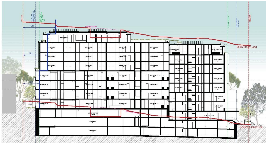
Figure 5: Section A with existing ground Line and recommended ADG setbacks shown over Source: Section MHNDU. Annotation Council staff
