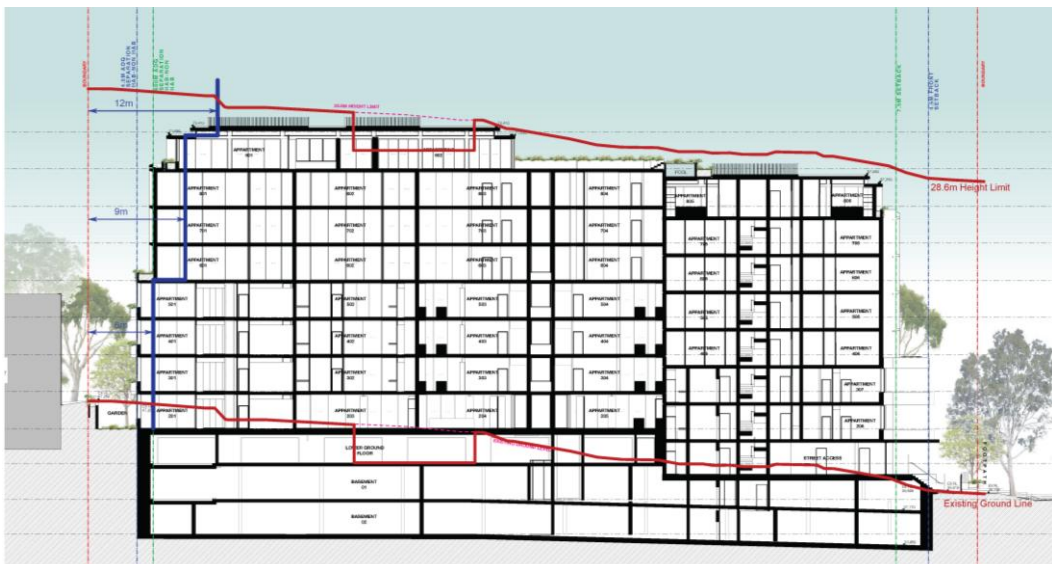
Figure 1 – Section A by MHNDU with existing ground Line and recommended ADG setbacks shown over
