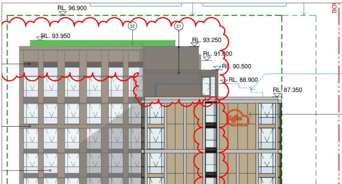
Figure 4: Proposed Amended Plan: North Elevation: DWG140 Rev I (additional height in green)
